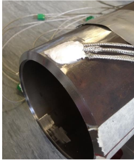
Figure 3-4 Protecting the tips of thermocouples on the outer surface by adhesive
