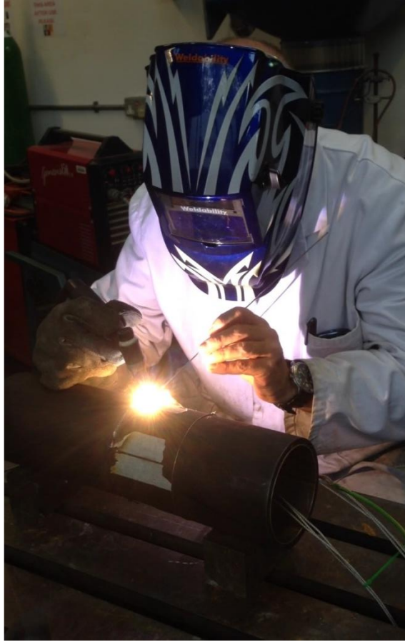
Figure 3-9 Lined pipe welding process using TIG welding
