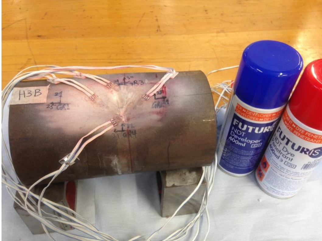
Figure 4-6 Using DPI penetrants to detect the surface-breaking cracks
