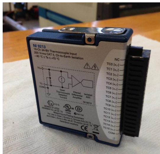
Figure A-1 Thermal module used to convert analogue signal to digital signal (ADC)
