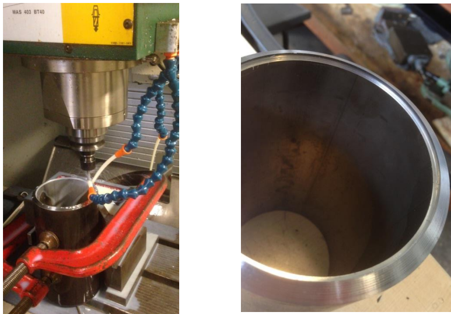
Figure 3-2 Cutting 3 mm from the liner and chamfering the edge of C-Mn by 30°
