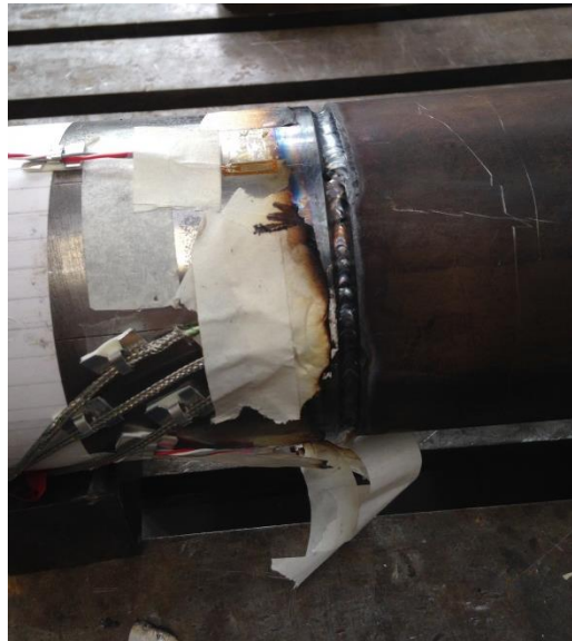
Figure 3-7 Measuring the temperatures and strains during welding
