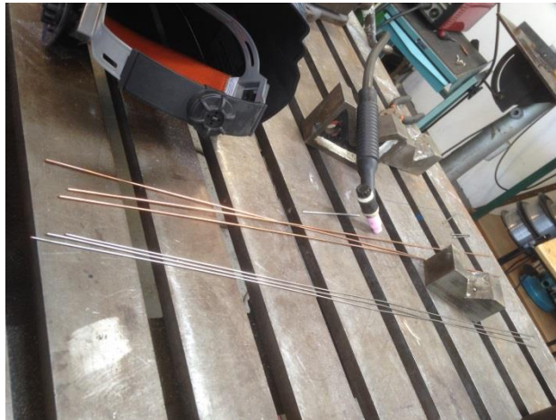
Figure 3-8 Rod types, E70S-2 (brass colour) and ER308L (grey colour)
