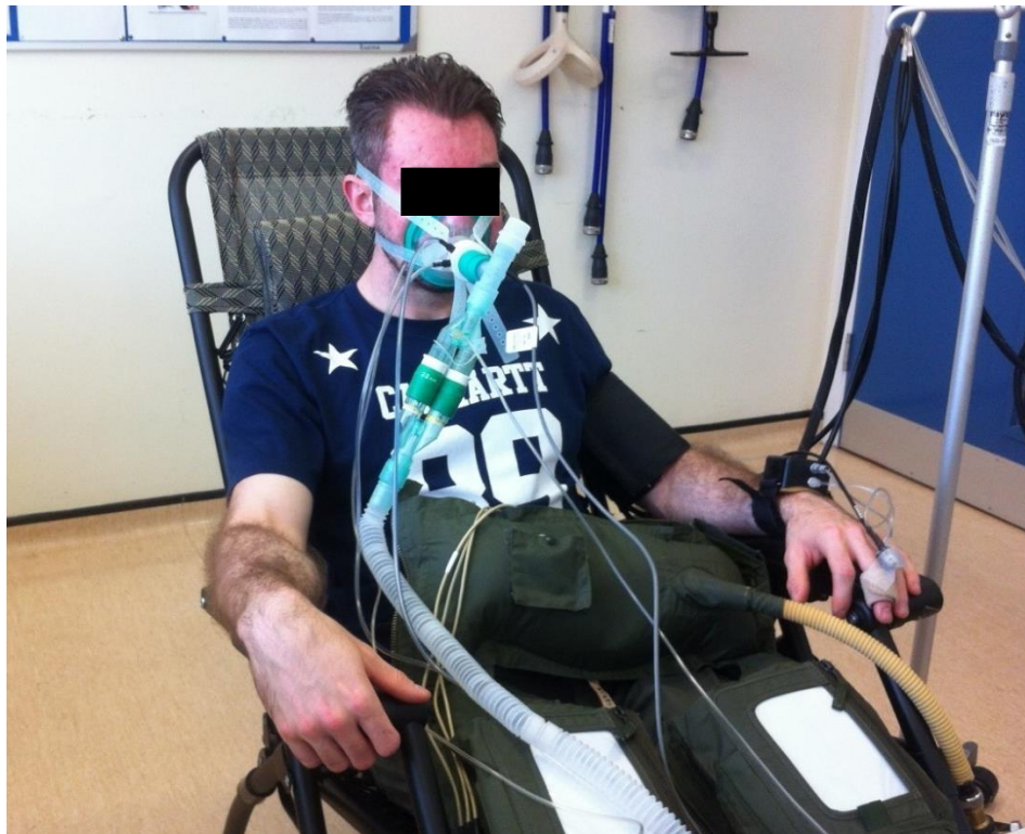
Figure 5-2 - Experimental set-up showing participant sitting in a semi-reclined chair while breathing against an inspiratory resistance and legs being compressed with anti-G trousers. The abdominal portion of the suit was kept loose to avoid compression of the abdomen.
