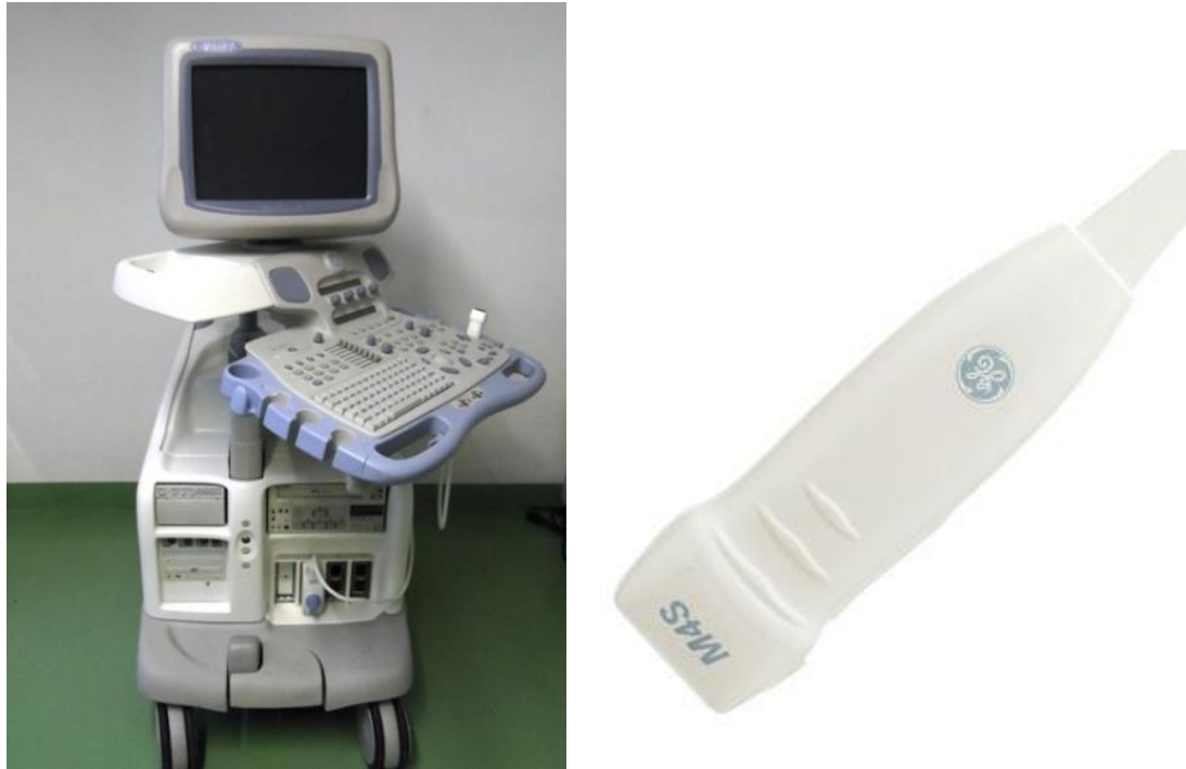
Figure 3-8 – Ultrasound system and probe. Images show (left panel) Vivid 7 ultrasound and (right panel) 2-D phased-array M4S transducer (both GE Medical, Horton, Norway) used in study 2 (Chapter 5).
