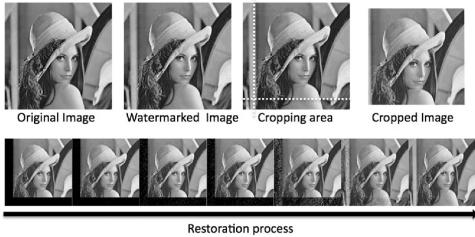
Fig. 5. Cropping-resistant tampering localisation and restoration performance of the proposed scheme. The original image, sized 256 \times 256 , was watermarked and then cropped to produce a 231 \times 231 image. The image was completely reconstructed.
