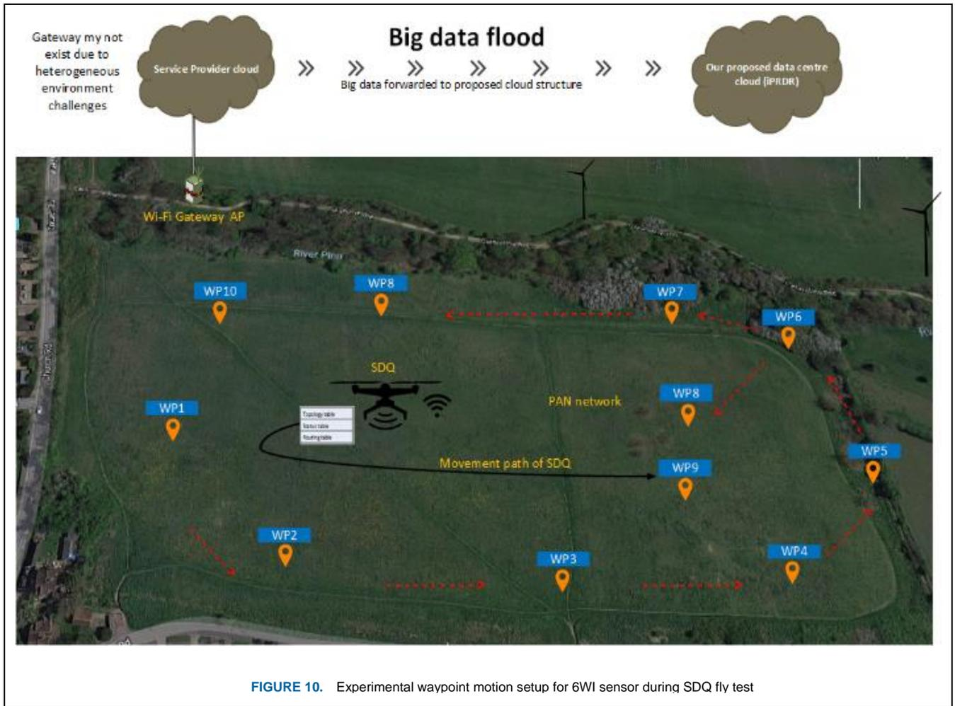
FIGURE 10. Experimental waypoint motion setup for 6WI sensor during SDQ fly test
