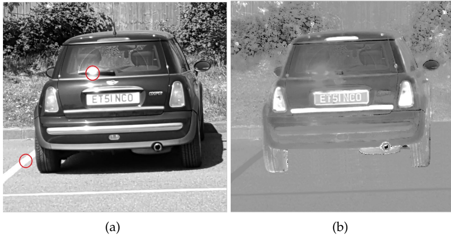
FIGURE 5.9: (a) The white paint and the white reflectance on the car have similar RGB values.(b) at C=0.21 the delta between these two regions becomes maximum. At this point Illumination Invariant image is produced where shadows and reflectance are removed.
