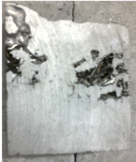
Figure 3.2: An attempt at producing a cuboidal specimen by pouring 650°C liquid A357 onto a heated fibre preform in a large, open mould with a rectangular cross-section. Very large voids are visible in the cross-section, which are the result of trapped air which caused the preform to float and required it to be manually held under the surface of the Al. The method was not pursued.
