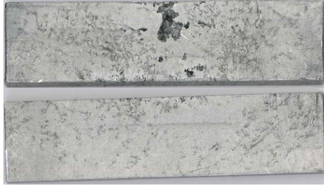
Figure 3.14: Smoothed cross-section of the induction-cast composite showing the distribution of fibres and shrinkage pores from the centre to the edge of the crucible.
