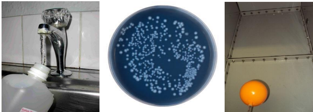
Figure 1.30a , Water sample collection for Legionella analysis in sterile bottles (supplied by UKAS accredited laboratory) in accordance with BS 7592:2008. Figure 1.30b , BCYE culture of Legionella bacteria from environmental water samples in UKAS accredited laboratory. Figure 1.30c , a sectional GRP tank after the cleaning and disinfection as water sample analysis of the stored water was identified with Legionella spp serogroup 1.
