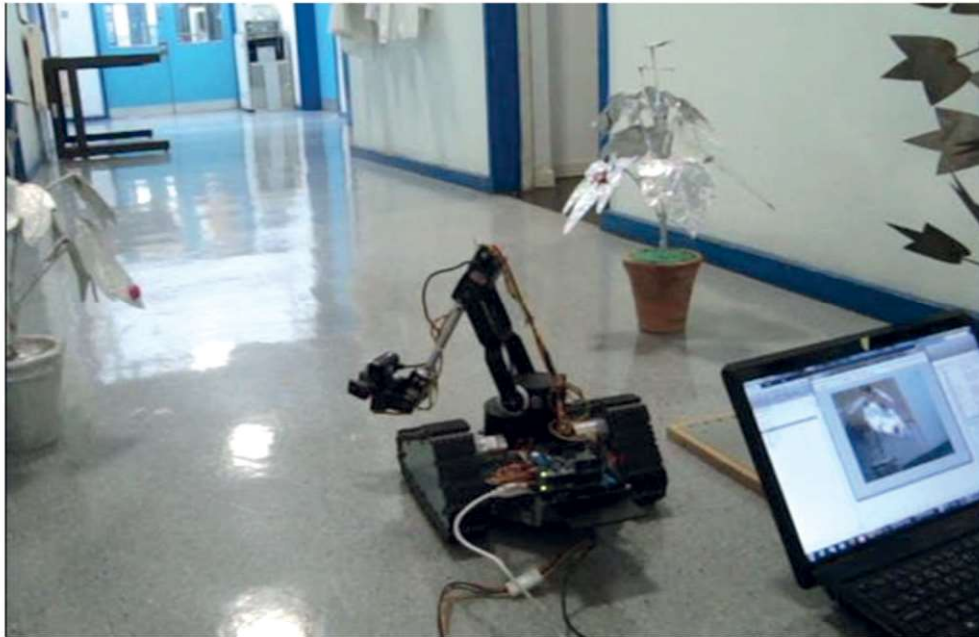
Figure 2: Induction electrostatic spray nozzle (IESN) installed on a mobile robotic arm with artificial plants along the path.
