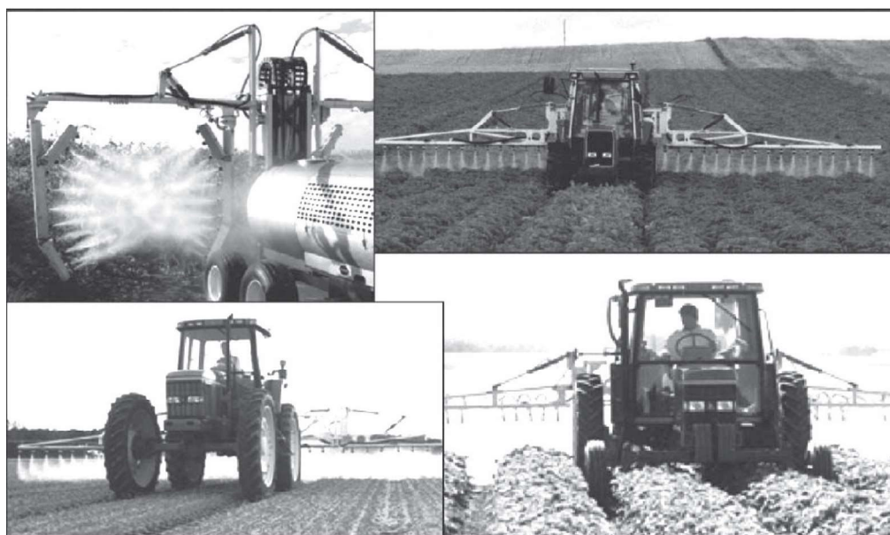
Figure 1: Electrostatic pesticide sprayer used in agricultural field (photos courtesy of Electrostatic Spraying Systems, Inc).
