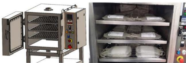
**Fig. 1.** a: 3D Render of Batch Freezer (b) Lab scale set up of Batch Freezer.
