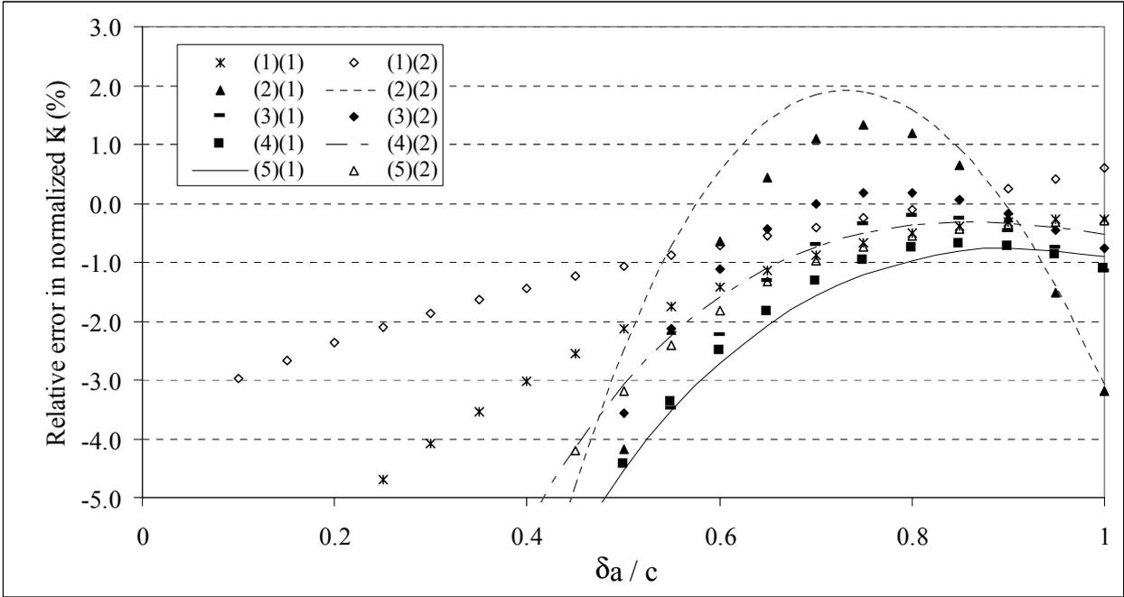
Figure 2: Relative error for the normalized stress intensity factor using several stress and displacements interpolating functions and  $0 < \delta a \leq c$ .
