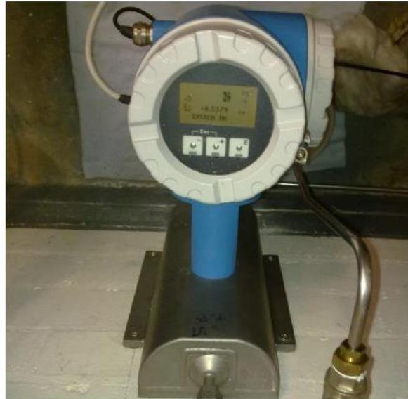
**Figure 18: E+H Promass 83 Coriolis Flow Meter**
