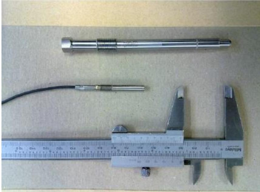
Figure 24: Kistler Pressure Transducer and Glow Plug Adapter
