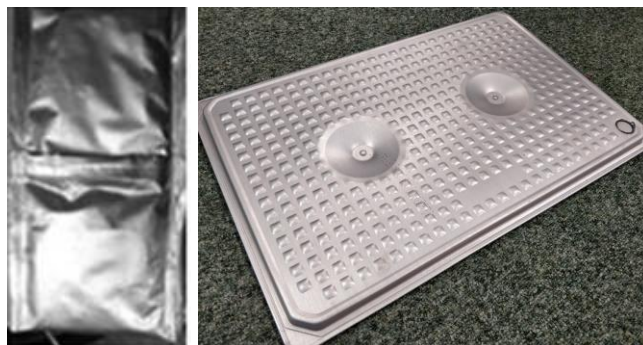
Figure 2.6 –Pouch and PCM panel used by Lazaro et al. (Lazaro, Dolado, Marín, et al., 2009; Lazaro, Dolado, Marin, et al., 2009)
