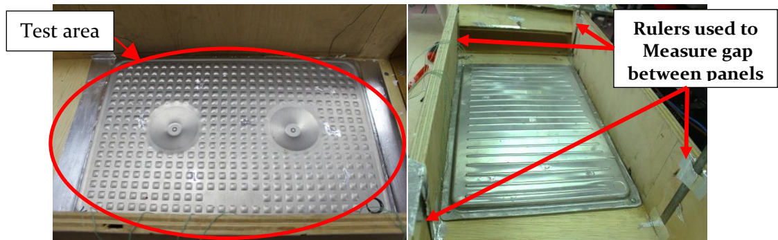
Figure 3.21 – Existing and new panels on the test rig with rulers used to measure the gap between panels.
