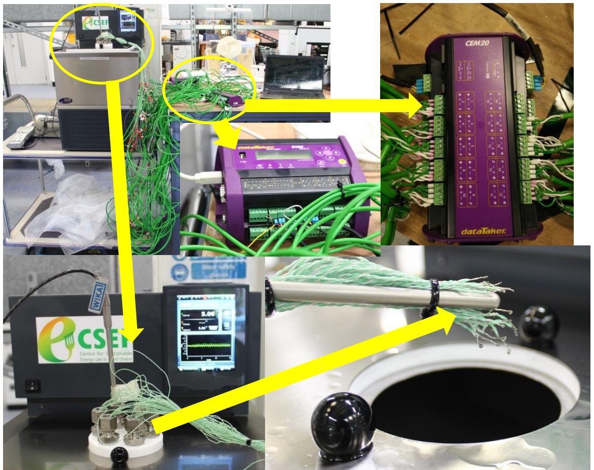
Figure VI.2 – Thermocouple calibration performed at CSEF with equipment used presented in detail.
