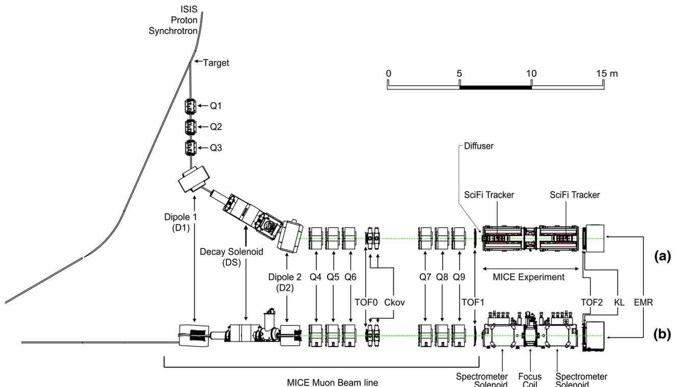
**Fig. 2** **a** Top and **b** side views of the MICE Muon Beam line, its instrumentation, and the experimental configuration. A titanium target dipped into the ISIS proton synchrotron and the resultant spill of particles was captured with a quadrupole triplet (Q1–3) and transported
