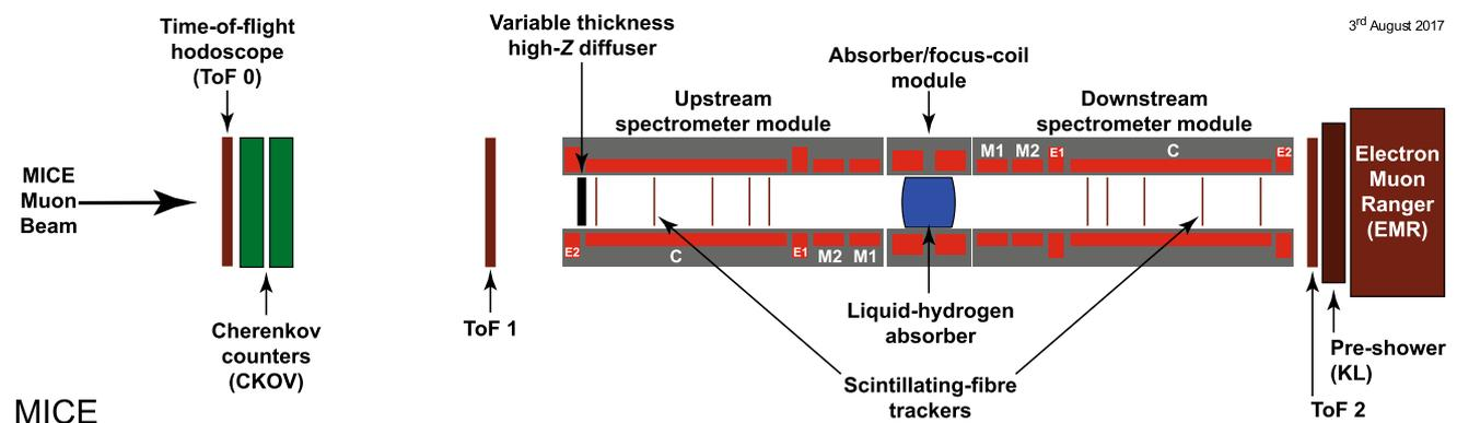
**Fig. 1** Schematic diagram of the MICE experiment. The red rectangles represent the coils of the spectrometer solenoids and focus-coil module. The individual coils of the spectrometer solenoids are labelled E1, C, E2, M1 and M2. The various detectors (time-of-flight hodoscopes
