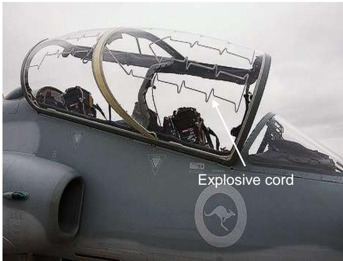
Figure 1.1 Photo showing the configuration of the linear explosive device bonded to a transparent canopy of an aircraft [2].
