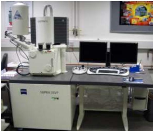
Figure 3.6 The photo of Zeiss Supra 35VP field-emission SEM equipped with EDS and EBSD detectors.
