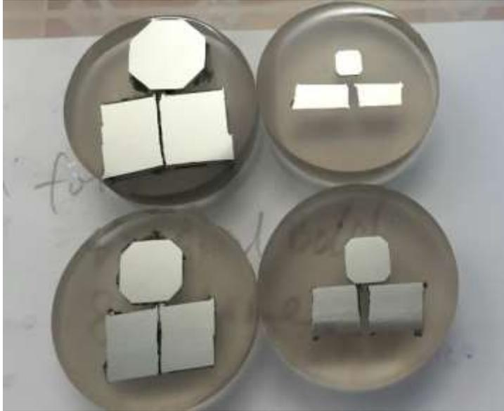
Figure 3.4 The photo of mounted specimens after polishing.
