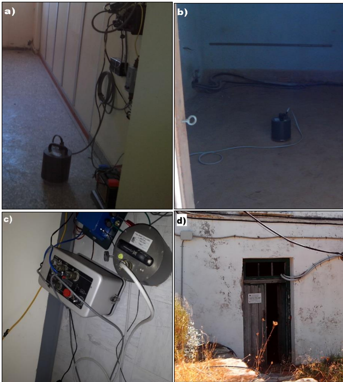
Figure 4.3.12. The HSNC sensors installed in empty of low anthropogenic activity building. Images from the TMBK(a), KNDR(b), CHAN(c) and KTHR(d) stations.
