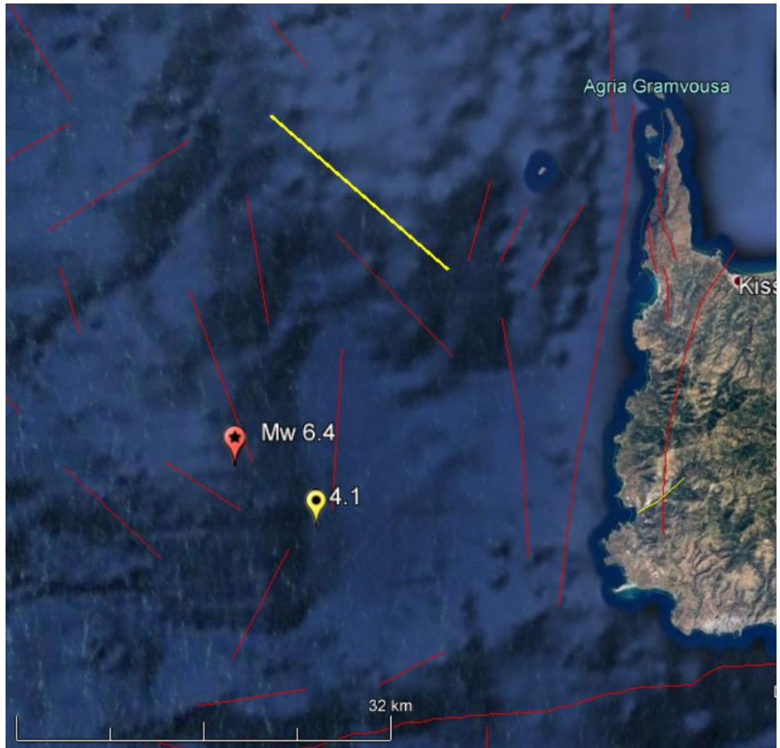
Figure 5.2.23 The registered faults in the NOA database (Ganas, et al., 2013) denoted with red lines while with yellows is likely the one that has been activated. The epicentres of the strong event of the 12/10/2013 sequence is marked with a red pin with a star and its largest aftershock is with the yellow pin (data processed in Google Earth (Google, 2018)).
