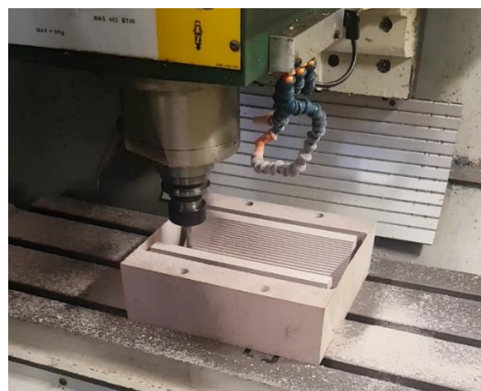
Figure 5.5. CNC machining in progress (CPC being milled in picture)
