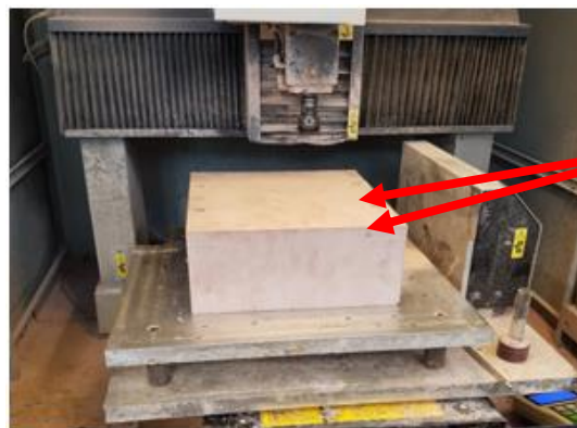
Figure 5.4. Setting up the Uriel on the CNC machine
