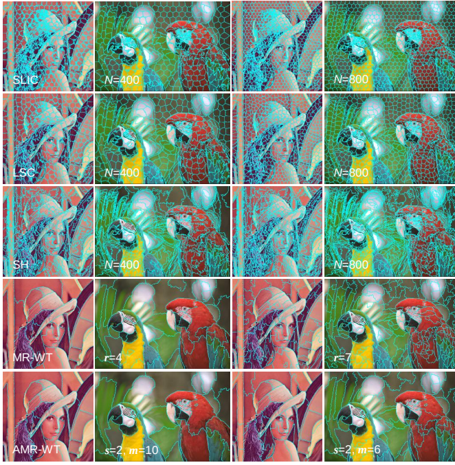
Fig. 12. Segmentation results on images with complex texture. Here, N denotes the number of superpixel areas used for SLIC, LSC, and SH; N is 400 for the left two images and N is 800 for the right two images. Also, r denotes the radius of structuring element used for MR-WT; values of r are 7 and 4, respectively. For AMR-WT, s = 2 and m = 10 are used for the left two images, while s = 2 and m = 6 are used for the right two images.
