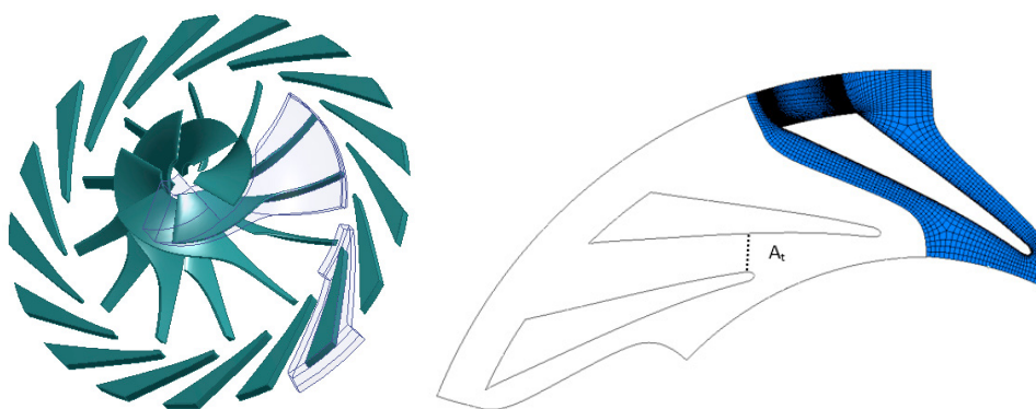
Fig. 1. Supercritical \text{CO}_2 compressor stage, the diffuser mesh by TurboGrid 17.1 and the throat area ( A_t ).
