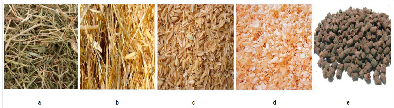
Fig. 1. Components of modelled chicken litter (a) hay, (b) straw, (c) rice husk, (d) wood shavings, (e) chicken manure.
