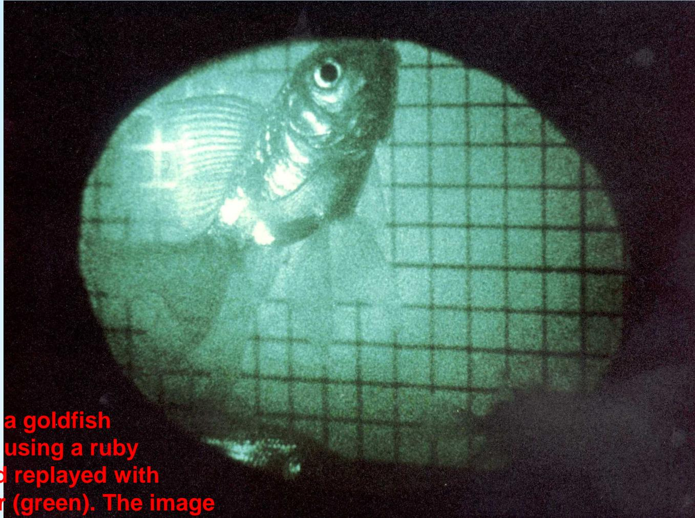
**This image of a goldfish was recorded using a ruby laser (red) and replayed with an argon laser (green). The image shows minimal aberrations.**
