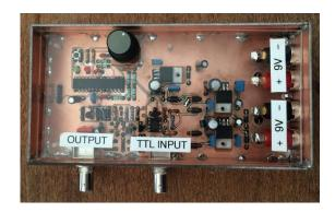
Figure 3.27: A professional precious power supply and oscillator
