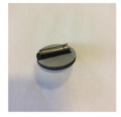
(e) Monuting the specimen on an aluminum pin stub
