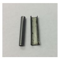
Figure 3.38: Comparison of mimicked stents before and after opening using handmade custom devices
