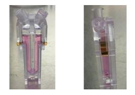
Figure 3.12: Zeta potential cuvette
