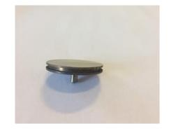
(a) An aluminium pin stub
