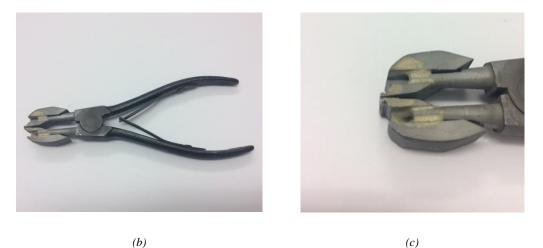
Figure 3.37: Two custom devices to open the stents: the linear wrench & holder (a) and the internal expanding gripper (b, c)
