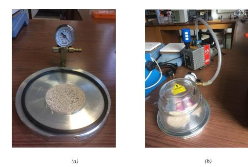
Figure 3.36: A petri dish of molecular sieve (a) and the sealed vacuum system for complete dryness of samples (b)
