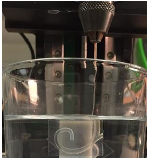
Figure 3-14. Before the insertion, the electrode array was clipped straight at the entry of the translucent cochlear model. It was placed in close proximity to the inner side wall.
