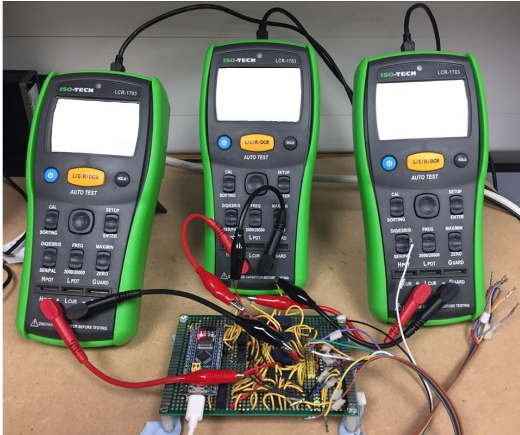
Figure 3-17: Three LCR Meters and a Channel Switchboard.
