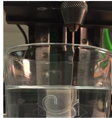
Fig. 4 Before the insertion, the electrode array was clipped straight at t entry of the translucent cochlear model. It was placed in close proximity to the inner side wall.
