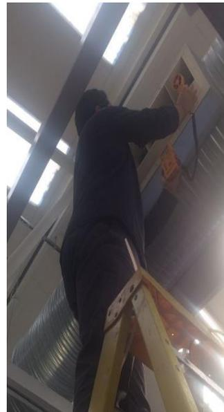
Figure 4.16 Measurements of air speed of the diffusers using CPS Thermo Anemometer AM
