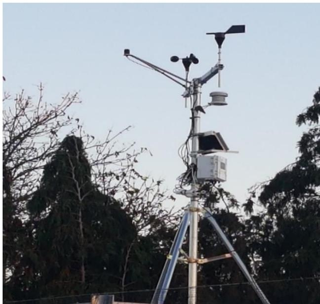
*Figure 4.12 U30-NRC-SYS-C HOBO Weather Station*
