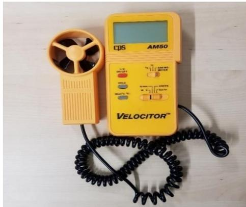
Figure 4.10 CPS Thermo Anemometer
