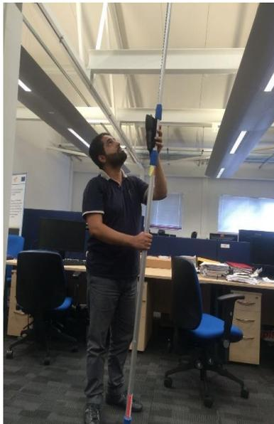
Figure 4.15 Measurements of mean air speed and temperature using a TA465 AirFlow instrument
