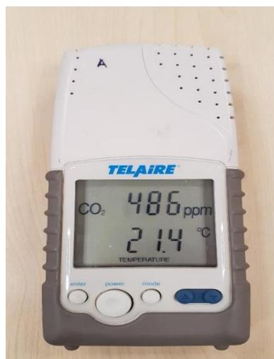
Figure 4.11 Telaire 7001 CO<sub>2</sub> Logger
