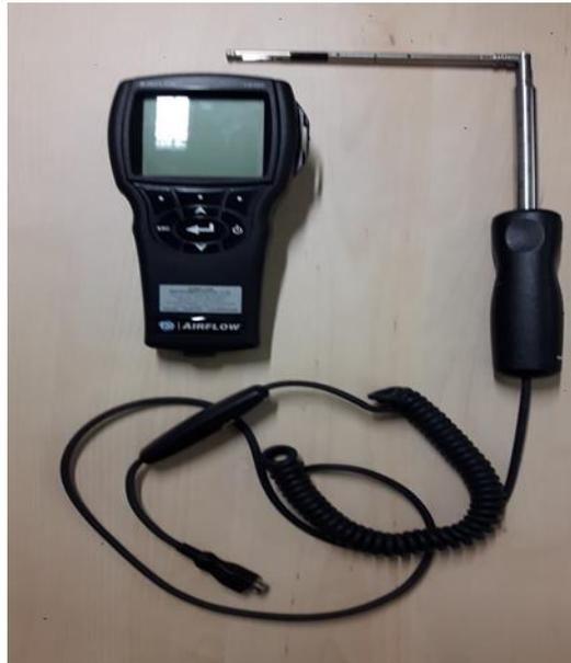
Figure 4.8 TA 465 AirFlow Instrument Air Velocity Meter
