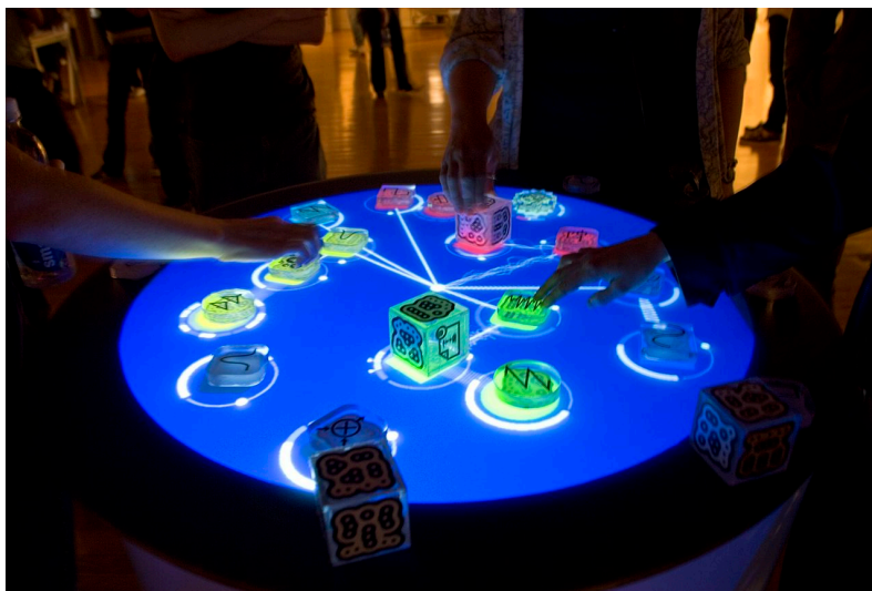
Fig. 2.4: Reactable, an electronic musical instrument with a tabletop Tangible User Interface (TUI) [Jor+07].
