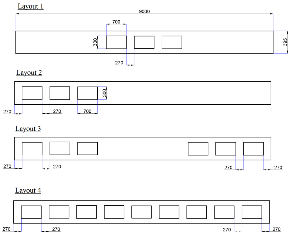
Fig. 7.8 Schematic of opening layout (all dimensions are in mm)
