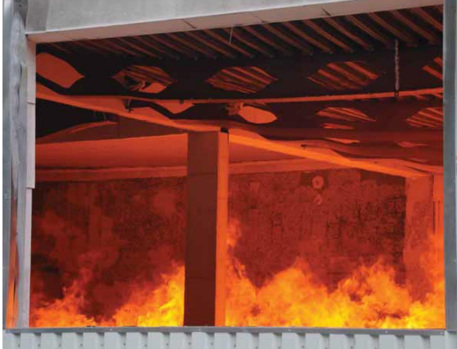
Fig. 2.14 Fire test on an administrative building in Mokrsko (Wald et al. 2011)
