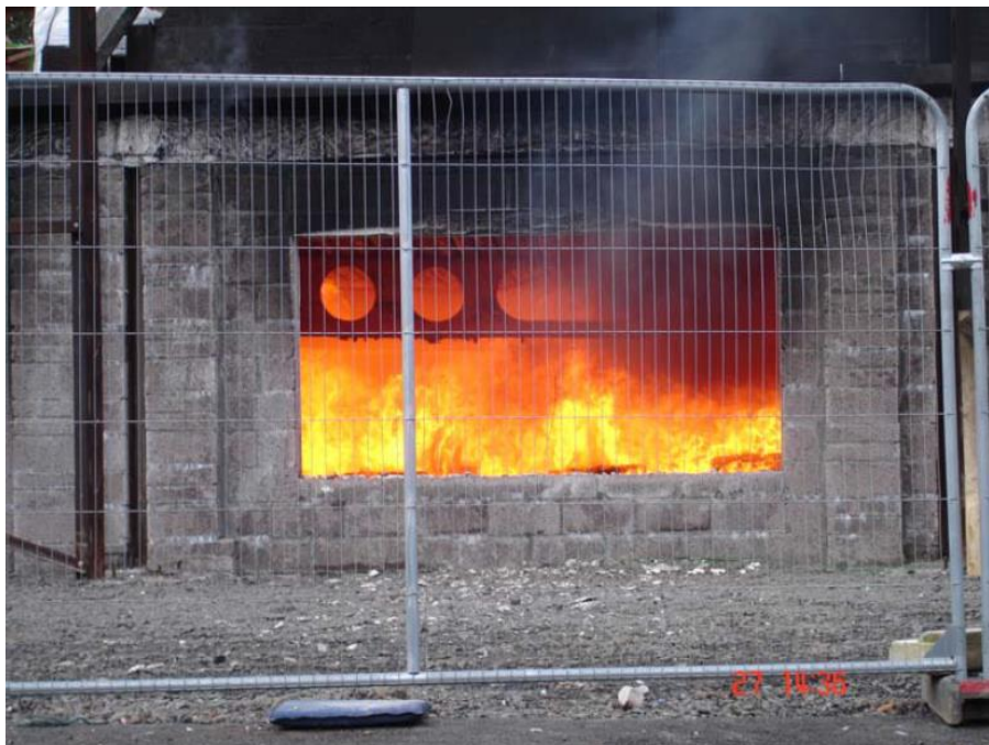
Fig. 2.15 Full-scale compartment test conducted at Ulster University (Nadjai et al. 2011)
