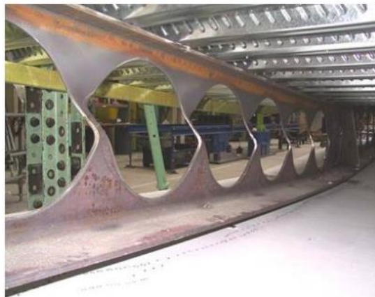
Fig. 2.12 Web-post buckling failure mode (Durif et al. 2013)
