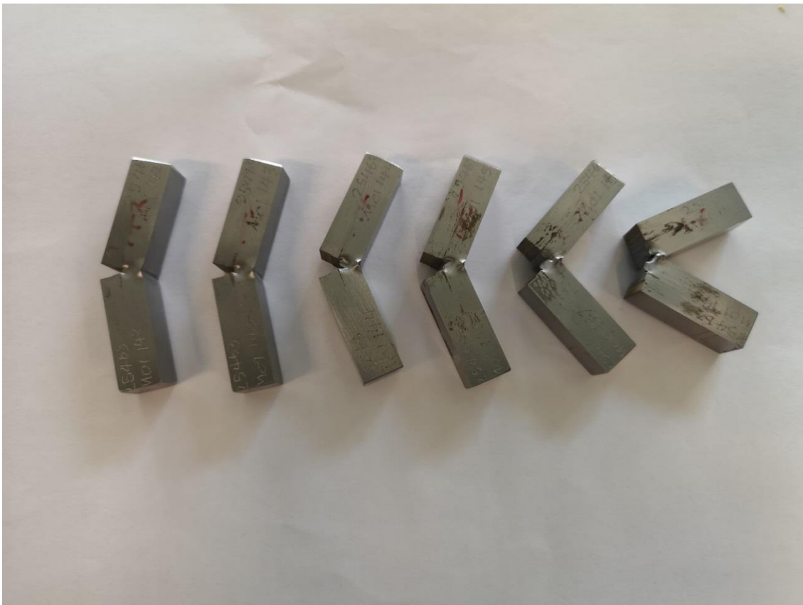
Figure 3.18 Low blow Instrumented pre-cracked Charpy tests at different angle of pendulum rise from 25° (LHS) to 40° (RHS) with 5° increments for S690QL.
