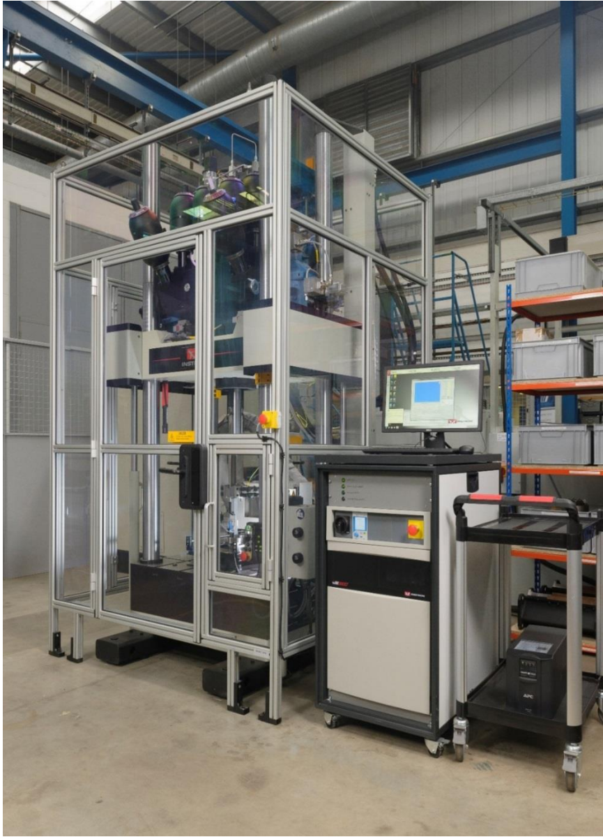
Figure 3.4 Instron VHS 160 dynamic test machine with capacity of 100 kN and speed up to 20 m/s. Courtesy of TWI Ltd.
