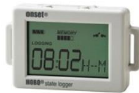
Figure 3.17: HOBO UX90-001M state/pulse/event/runtime data logger
