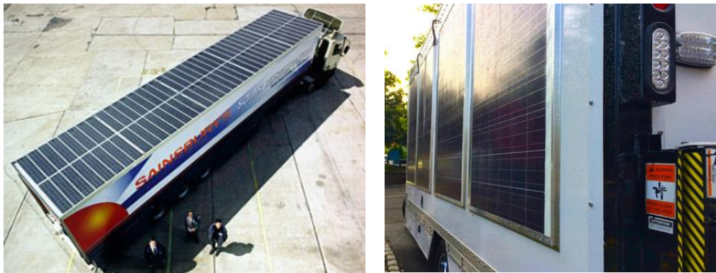
Figure 2.8: Solar-powered transport refrigeration
