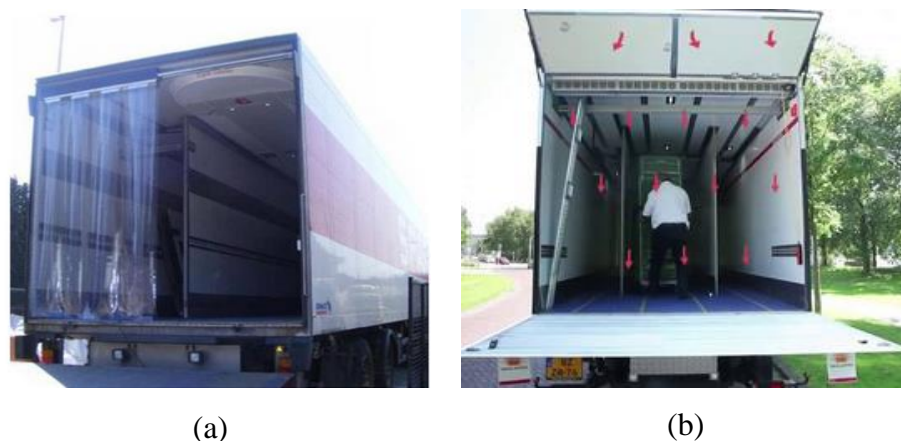
Figure 2.5: Protective mechanisms (a) PVC strip curtain and (b) air curtain.
