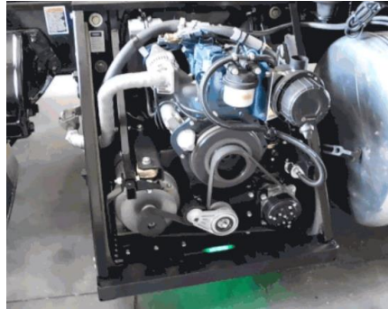
Figure 3.2: 4.0 kW auxiliary diesel engine [75].
