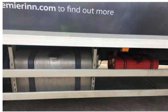
Figure 2.4: Main engine tank for white diesel and auxiliary engine tank for red diesel.
