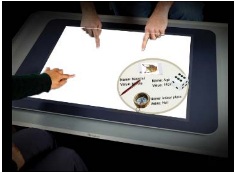
Figure 2. A sketch envisioning the tactile paradigm: a smart card depicting an ancient vase is on the tabletop and a set of tangible attributes are in the smart card area in order to associate some attributes.
