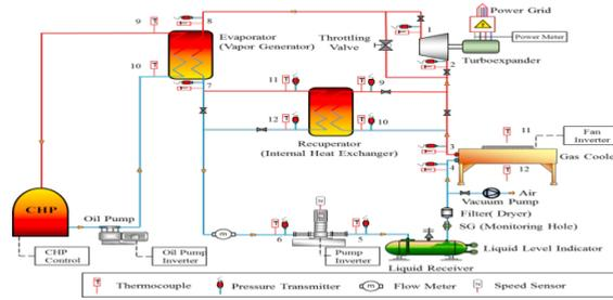
Fig. 1. Process flow diagram with the relative sensors position of a recuperative ORC test rig.
