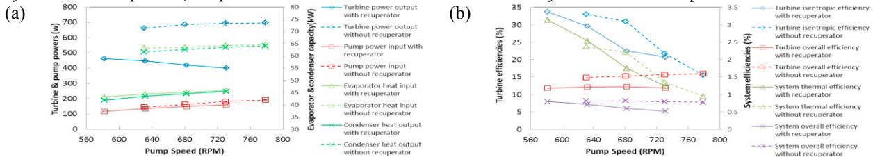
Fig. 6. Variations of turbine and pump powers and evaporator and condenser capacities (a) and turbine and system efficiencies (b) with ORC pump speeds on system with and without recuperator.
