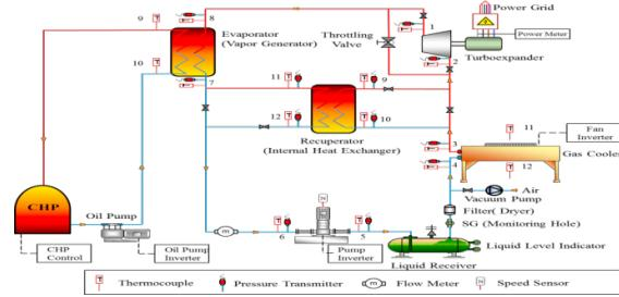
Fig. 1. Process flow diagram with the relative sensors position of a recuperative ORC test rig.
