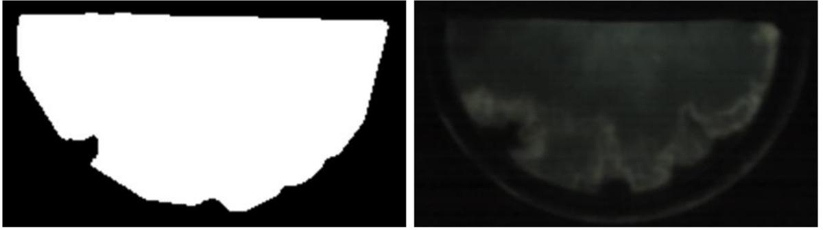
Figure 4.6 Raw combustion image (right) and binary image following the mask filter (left)
