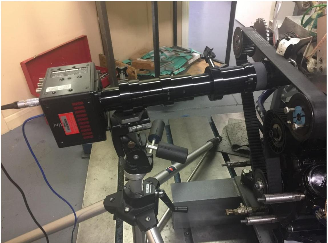
Figure 8.14 *FastCam* mini with telescope
