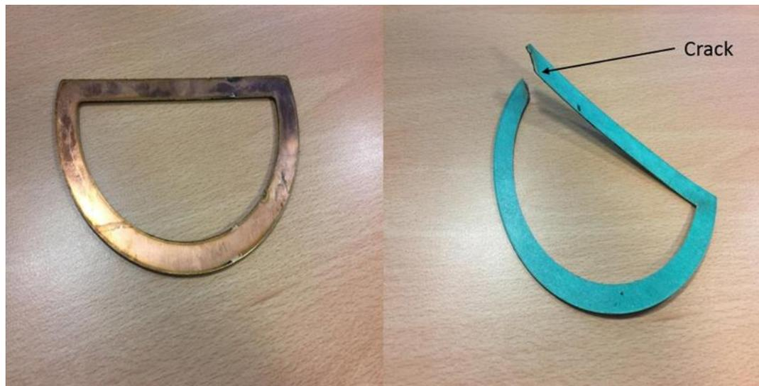
Figure 5.3 Copper top window gasket (left) and paper gasket (right)
