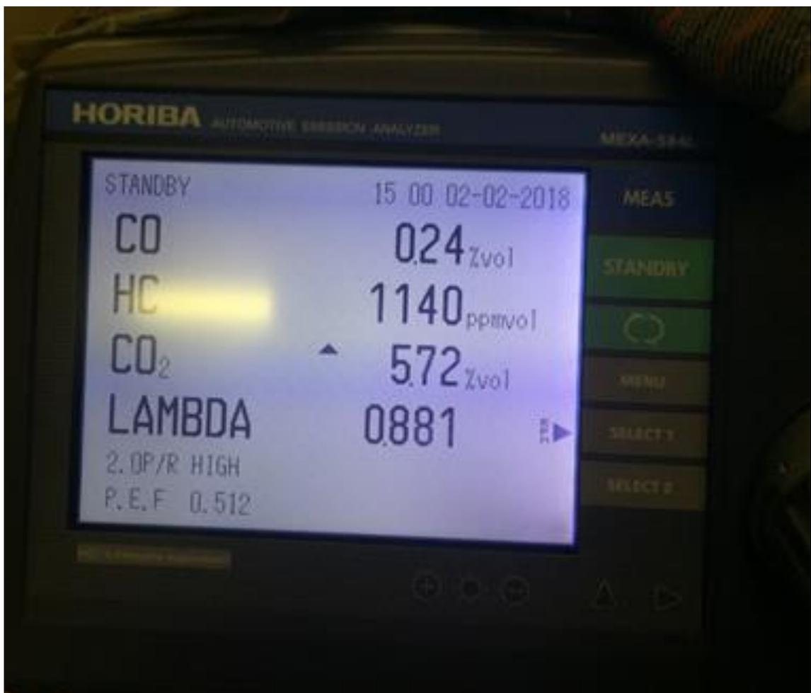
Figure 3.24 Photo of MEXA-584L gas analyser
