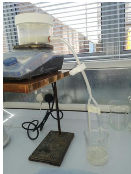
Figure 3-7 Calcium alginate-Pyrax clay beads preparation apparatus
