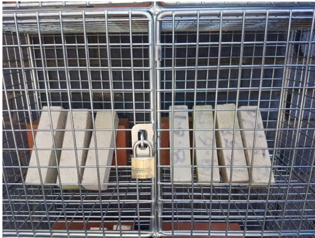
Figure 9-1 Outdoor Exposure (wire shelving unit) Figure 9-2 Samples were positioned 45°
