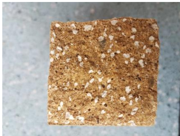
Figure 6-7 Mortar specimen contain 7% of cement weight calcium alginate-pyrophyllite beads
