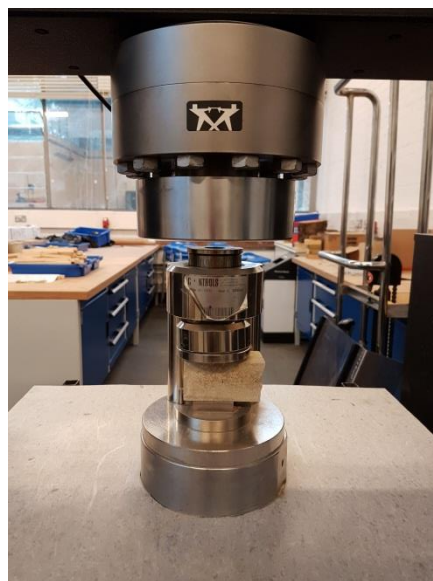
Figure 3-9 Instron Universal Machine (UTM) for compressive strength test
