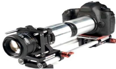
**Figure 1.** Holoscopic 3D camera prototype by 3DVIVANT project at Brunel University London [20].
