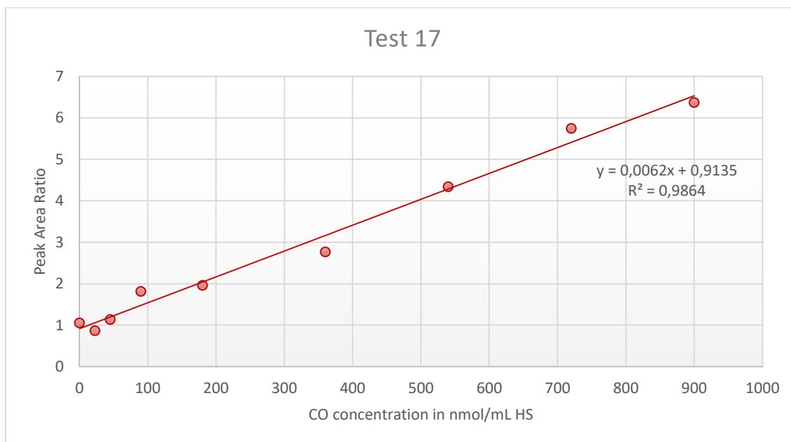
**Figure A3.17:** Peak Area Ratio of carbon monoxide (CO) from the blood sample over  $^{13}\text{CO}$  from the internal standard (IS) plotted against the CO concentration in the calibration standards, with addition of linear trendline, linear regression equation and regression coefficient ( $R^2$ ) for Test 17.
