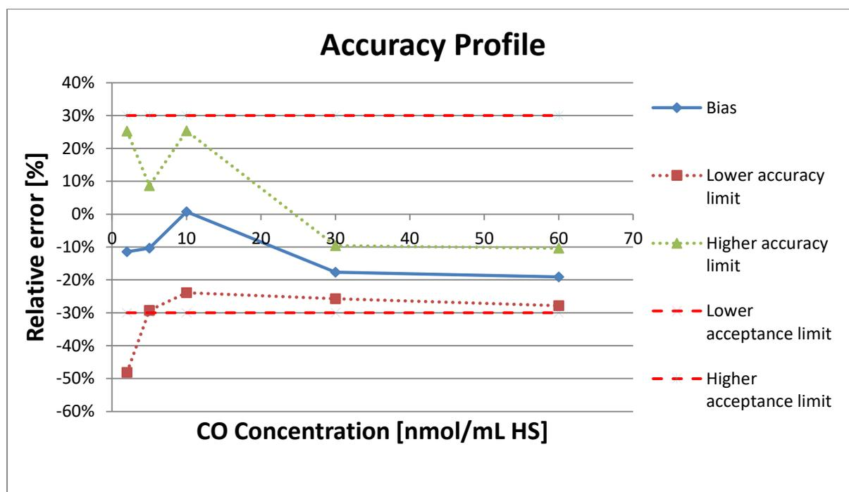
**Figure 3.4:** Accuracy profile for CO determination using a simple linear regression model within the range of 2-60 nmol/mL HS (0.8-24  $\mu$ mol/mL blood). The continuous line represents the trueness (bias), the dashed lines represent the acceptance limits set at  $\pm 30\%$  and the dotted lines are the relative lower and upper accuracy limits.
