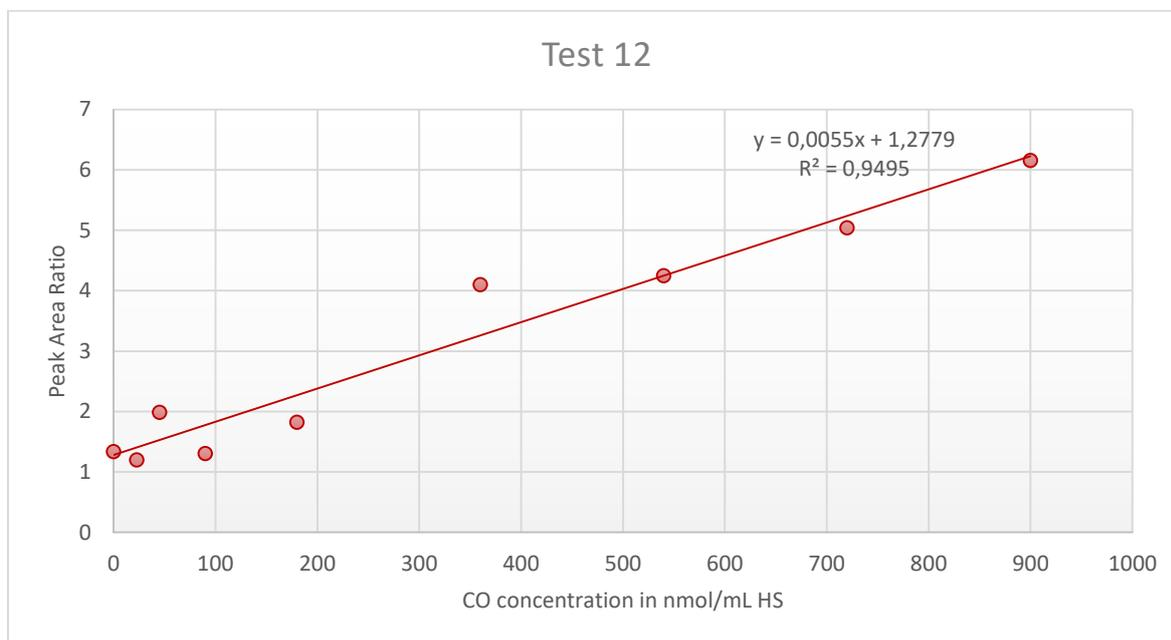
**Figure A3.12:** Peak Area Ratio of carbon monoxide (CO) from the blood sample over  $^{13}\text{CO}$  from the internal standard (IS) plotted against the CO concentration in the calibration standards, with addition of linear trendline, linear regression equation and regression coefficient ( $R^2$ ) for Test 12.
