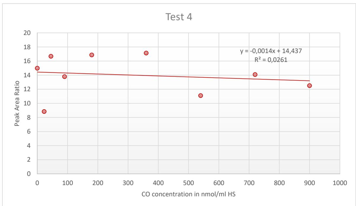
**Figure A3.4:** Peak Area Ratio of carbon monoxide (CO) from the blood sample over  $^{13}\text{C}$ O from the internal standard (IS) plotted against the CO concentration in the calibration standards, with addition of linear trendline, linear regression equation and regression coefficient ( $R^2$ ) for Test 4.
