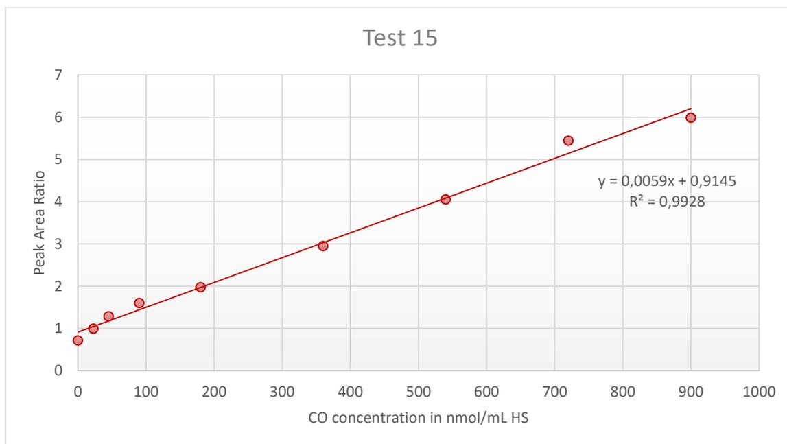
**Figure A3.15:** Peak Area Ratio of carbon monoxide (CO) from the blood sample over  $^{13}\text{C}$ CO from the internal standard (IS) plotted against the CO concentration in the calibration standards, with addition of linear trendline, linear regression equation and regression coefficient ( $R^2$ ) for Test 15.
