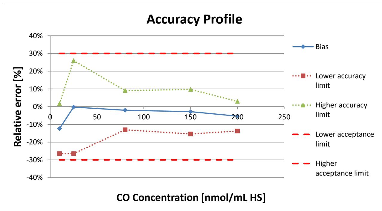
**Figure 3.2:** Accuracy profile for CO determination using a simple linear regression model within the range of 10-200 nmol/mL HS (2-40  $\mu\text{mol/mL}$  blood). The continuous line represents the trueness (bias), the dashed lines represent the acceptance limits set at  $\pm 30\%$  and the dotted lines are the relative lower and upper accuracy limits.
