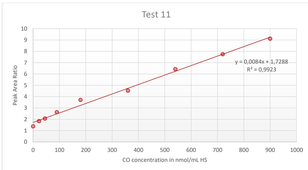
**Figure A3.11:** Peak Area Ratio of carbon monoxide (CO) from the blood sample over  $^{13}\text{CO}$  from the internal standard (IS) plotted against the CO concentration in the calibration standards, with addition of linear trendline, linear regression equation and regression coefficient ( $R^2$ ) for Test 11.
