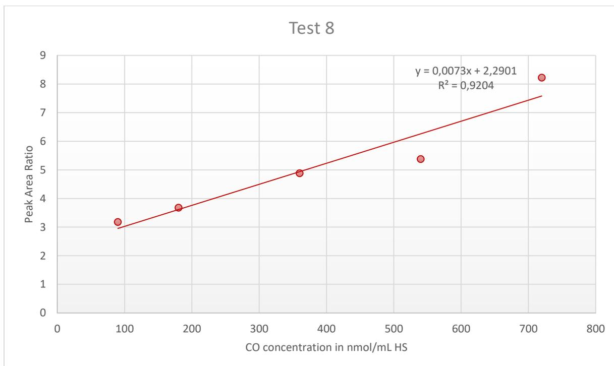
**Figure A3.8:** Peak Area Ratio of carbon monoxide (CO) from the blood sample over  $^{13}\text{C}$ CO from the internal standard (IS) plotted against the CO concentration in the calibration standards, with addition of linear trendline, linear regression equation and regression coefficient ( $R^2$ ) for Test 8.
