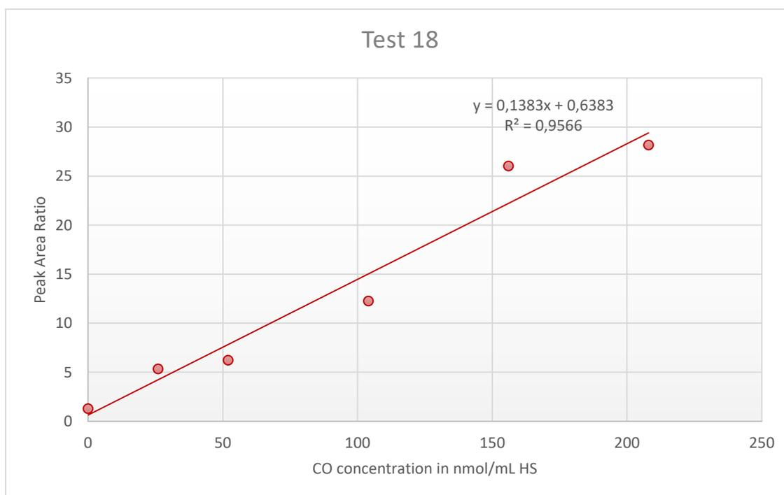
**Figure A3.18:** Peak Area Ratio of carbon monoxide (CO) from the blood sample over  $^{13}\text{CO}$  from the internal standard (IS) plotted against the CO concentration in the calibration standards, with addition of linear trendline, linear regression equation and regression coefficient ( $R^2$ ) for Test 18.
