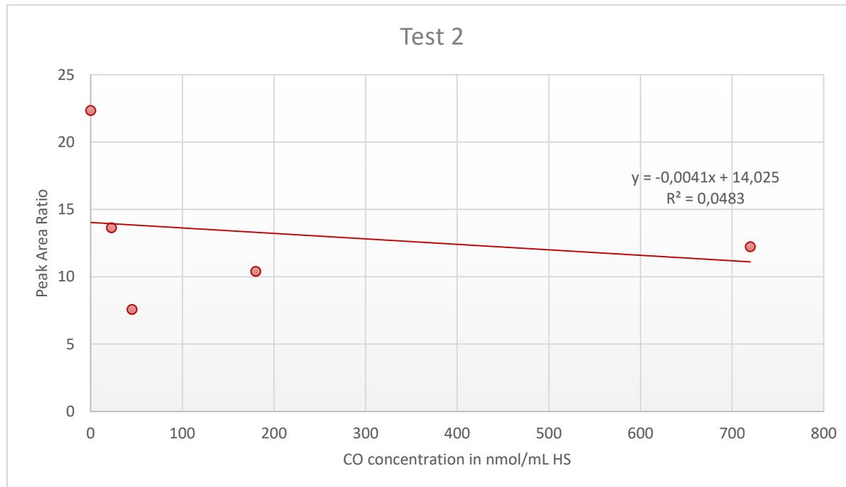
**Figure A3.2:** Peak Area Ratio of carbon monoxide (CO) from the blood sample over  $^{13}\text{C}$ O from the internal standard (IS) plotted against the CO concentration in the calibration standards, with addition of linear trendline, linear regression equation and regression coefficient ( $R^2$ ) for Test 2.
