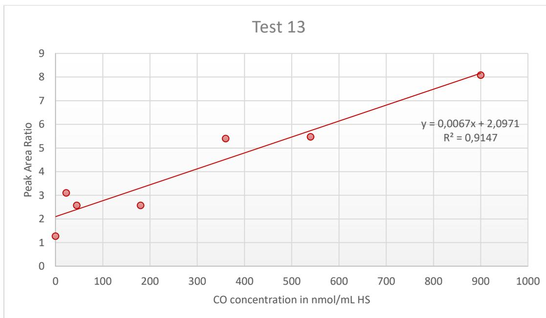
**Figure A3.13:** Peak Area Ratio of carbon monoxide (CO) from the blood sample over  $^{13}\text{CO}$  from the internal standard (IS) plotted against the CO concentration in the calibration standards, with addition of linear trendline, linear regression equation and regression coefficient ( $R^2$ ) for Test 13.
