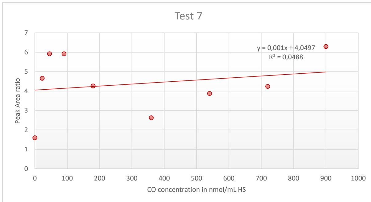
**Figure A3.7:** Peak Area Ratio of carbon monoxide (CO) from the blood sample over  $^{13}\text{C}$ CO from the internal standard (IS) plotted against the CO concentration in the calibration standards, with addition of linear trendline, linear regression equation and regression coefficient ( $R^2$ ) for Test 7.
