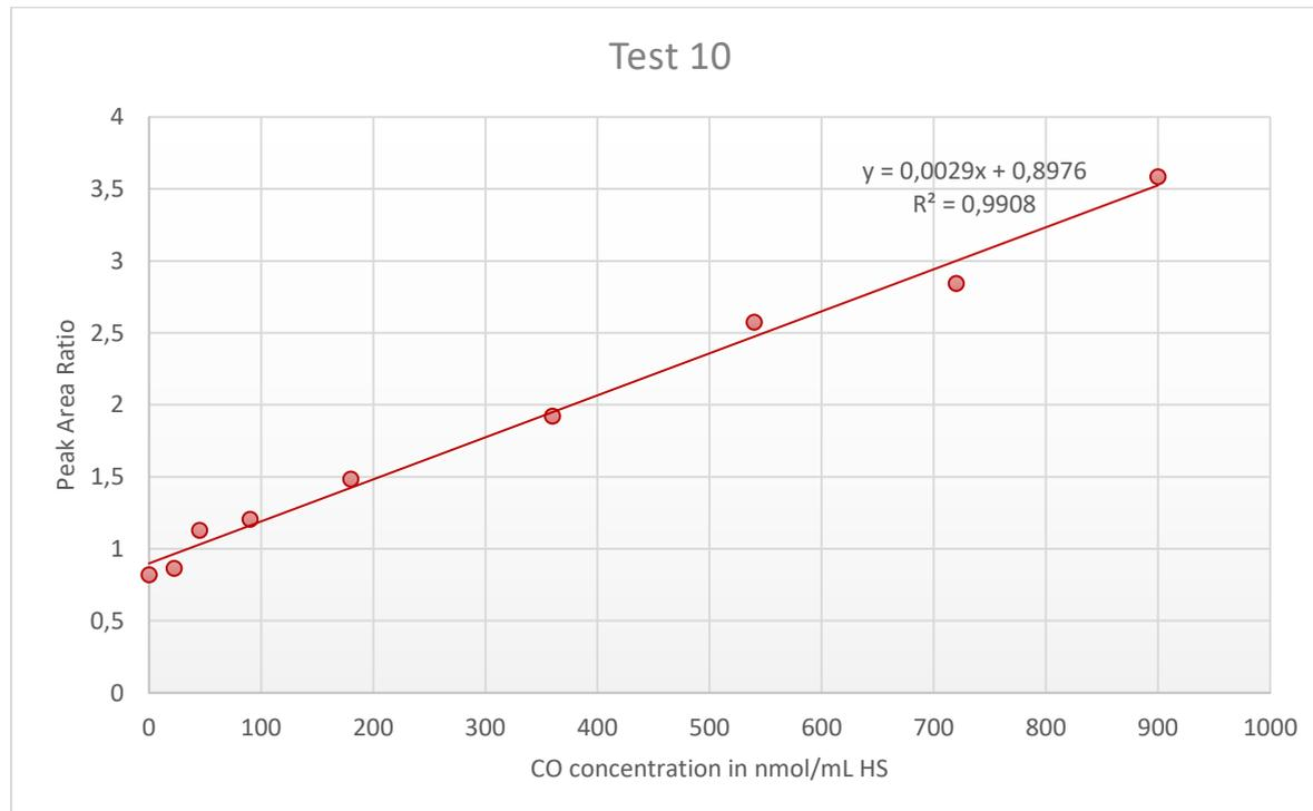
**Figure A3.10:** Peak Area Ratio of carbon monoxide (CO) from the blood sample over  $^{13}\text{C}$ CO from the internal standard (IS) plotted against the CO concentration in the calibration standards, with addition of linear trendline, linear regression equation and regression coefficient ( $R^2$ ) for Test 10.
