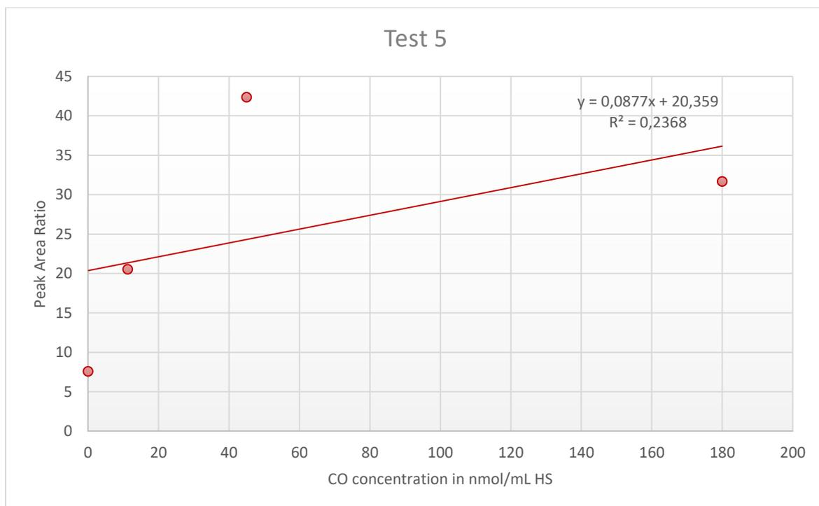
**Figure A3.5:** Peak Area Ratio of carbon monoxide (CO) from the blood sample over  $^{13}\text{C}$ CO from the internal standard (IS) plotted against the CO concentration in the calibration standards, with addition of linear trendline, linear regression equation and regression coefficient ( $R^2$ ) for Test 5.
