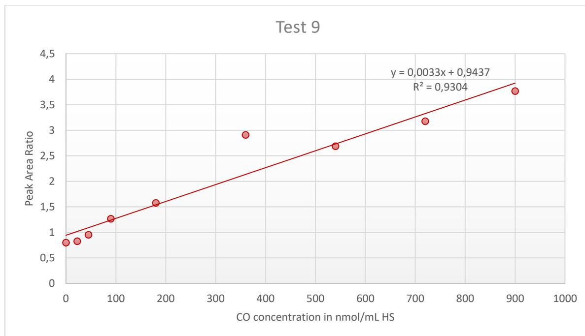
**Figure A3.9:** Peak Area Ratio of carbon monoxide (CO) from the blood sample over  $^{13}\text{C}$ CO from the internal standard (IS) plotted against the CO concentration in the calibration standards, with addition of linear trendline, linear regression equation and regression coefficient ( $R^2$ ) for Test 9.
