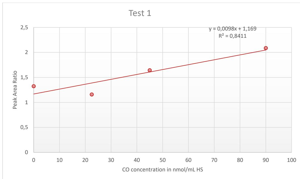
**Figure A3.1:** Peak Area Ratio of carbon monoxide (CO) from the blood sample over  $^{13}\text{C}$ O from the internal standard (IS) plotted against the CO concentration in the calibration standards, with addition of linear trendline, linear regression equation and regression coefficient ( $R^2$ ) for Test 1.
