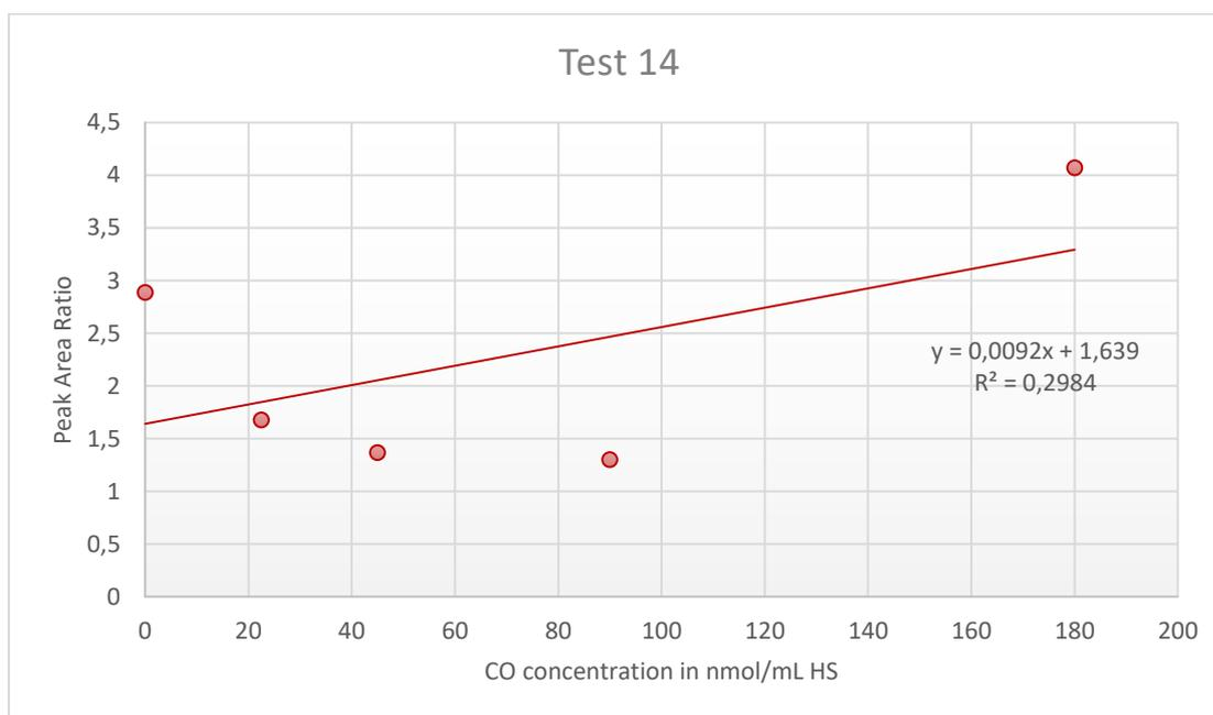
**Figure A3.14:** Peak Area Ratio of carbon monoxide (CO) from the blood sample over  $^{13}\text{CO}$  from the internal standard (IS) plotted against the CO concentration in the calibration standards, with addition of linear trendline, linear regression equation and regression coefficient ( $R^2$ ) for Test 14.
