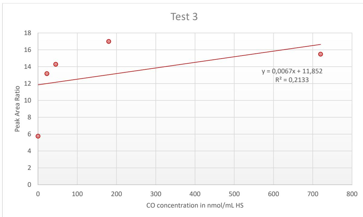
**Figure A3.3:** Peak Area Ratio of carbon monoxide (CO) from the blood sample over  $^{13}\text{C}$ O from the internal standard (IS) plotted against the CO concentration in the calibration standards, with addition of linear trendline, linear regression equation and regression coefficient ( $R^2$ ) for Test 3.
