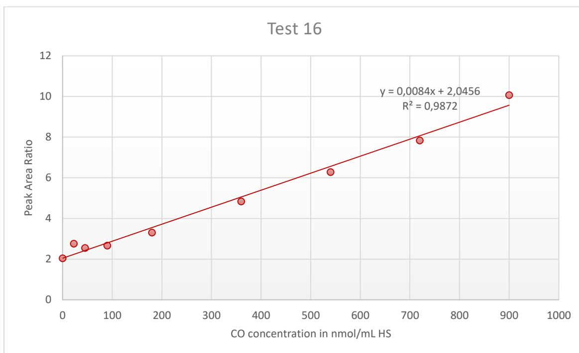
**Figure A3.16:** Peak Area Ratio of carbon monoxide (CO) from the blood sample over  $^{13}\text{C}$ CO from the internal standard (IS) plotted against the CO concentration in the calibration standards, with addition of linear trendline, linear regression equation and regression coefficient ( $R^2$ ) for Test 16.
