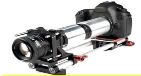
Figure 3.16: Holoscopic 3D camera prototype by 3DVJVANT project at Brunel University. [81].
