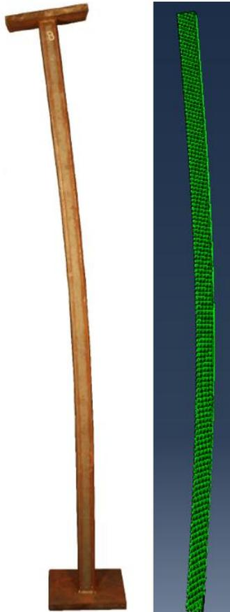
Figure 3.25: Test and FE failure mode of S355 beam-column member level, RHS 120x60x3.6-
