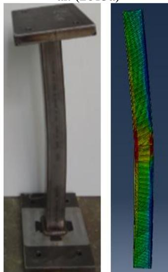
Figure 3.19: Test and FE failure mode beam-columns SHS 60×60×3,  $e_z=10\text{mm}$ . Test from Zhao et al. (2016b)
