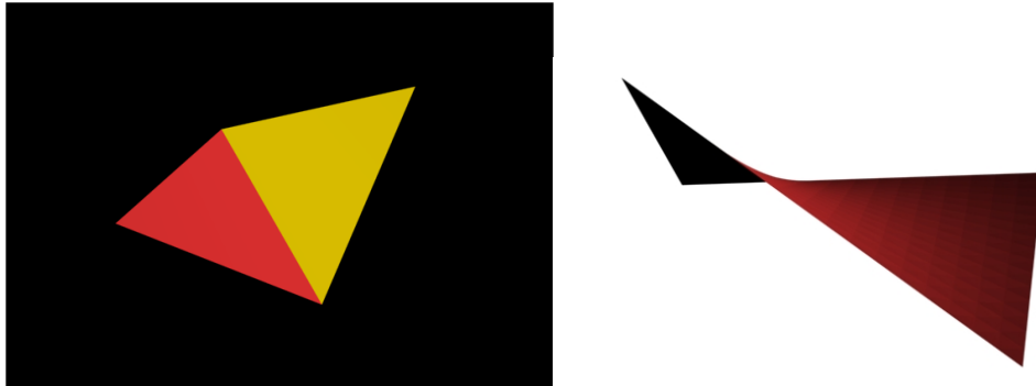
Figure 118. Reconstructing stratigraphic surfaces from four theodolite-recorded points; i) The interface is rendered as two separate flat polygons ii) approximated by a NURBS surface.
