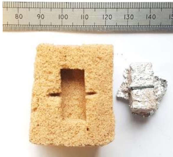
Figure 3-1- Sand mould and the aluminium-zinc coated steel overcast. Sand moulds with similar dimensions were used for all of the experiments.
