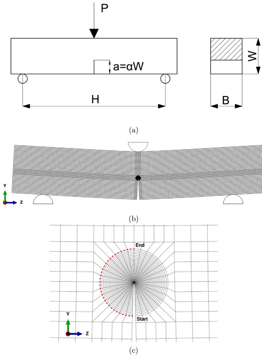
Fig. 1. Three-point SENB specimen - SENB: (a) schematic drawing, (b) finite element model of SENB with  $\alpha = 0.45$  (see also Table 1), (c) crack tip zone with highlighted path for strain extraction.
