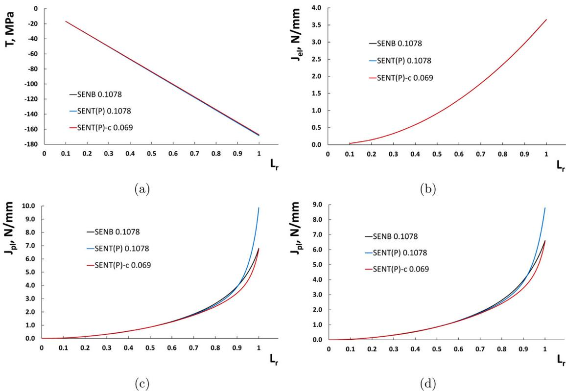
Fig. 11. SENB-SENT(P) shallow cracks. (a)  $T$ -stress values at limit load (b)  $J_{el}$  values at limit load (c)  $J_{pl}$  values at limit load using EPP material model (d)  $J_{pl}$  values at limit load using EPH material model.
