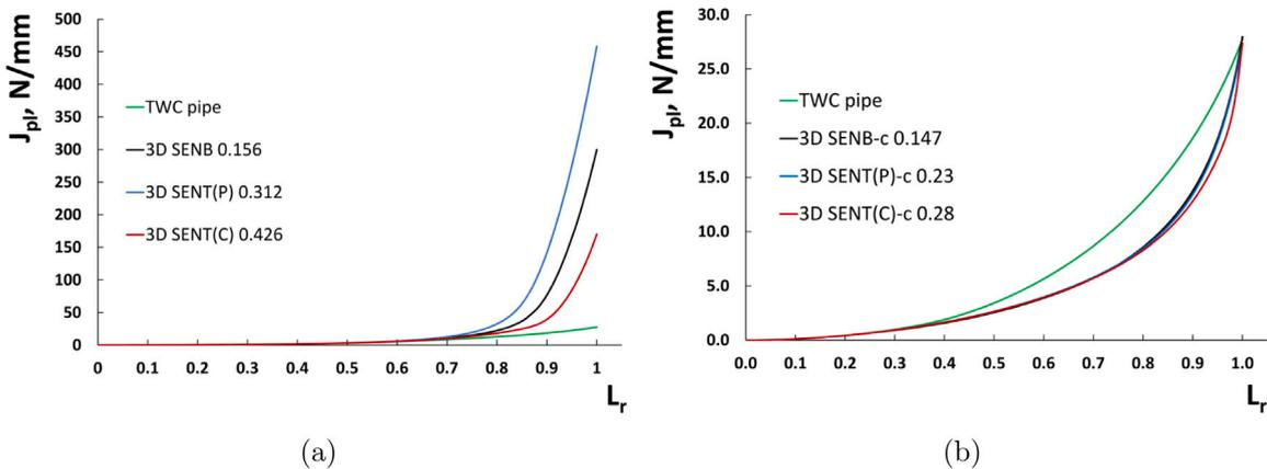
**Fig. 16.** TWC pipe and 3D specimens using EPH material option: (a) 3D specimens subjected to plane strain limit loads (b) 3D samples subjected to corrected plane strain limit loads.
