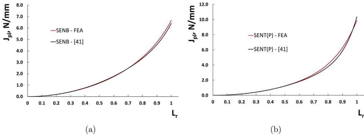
Fig. 7. Comparison of finite element results with EPRI procedure: (a) SENB sample with  $\alpha = 0.25$ , (b) SENT(P) sample with  $\alpha = 0.25$ .
