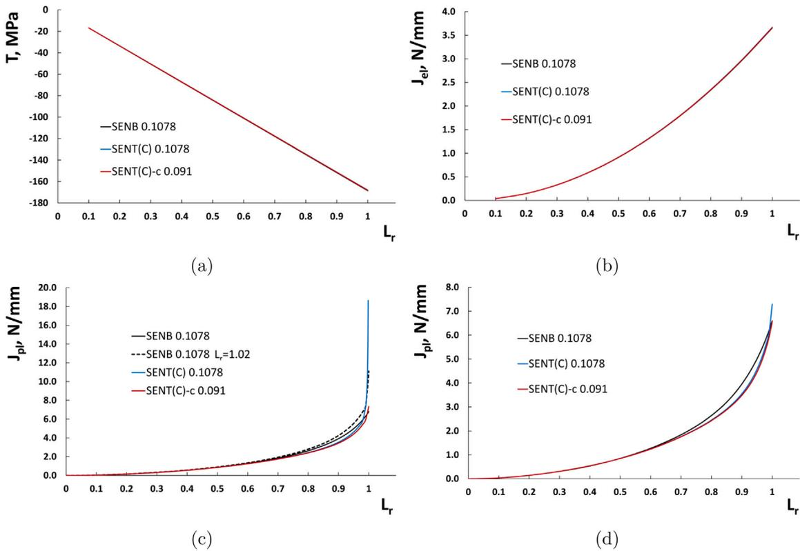
Fig. 9. SENB-SENT(C) matching for shallow cracks. (a)  $T$ -stress values at limit load (b)  $J_{el}$  values at limit load (c)  $J_{pl}$  values at limit load using EPP material model (d)  $J_{pl}$  values at limit load using EPH material model.
