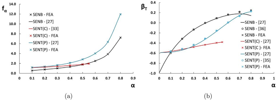
Fig. 5. Comparison of results from elastic finite element analyses with solutions from the literature [27,33,35,36]: (a) normalised stress intensity factor, (b) normalised constraint parameter.
