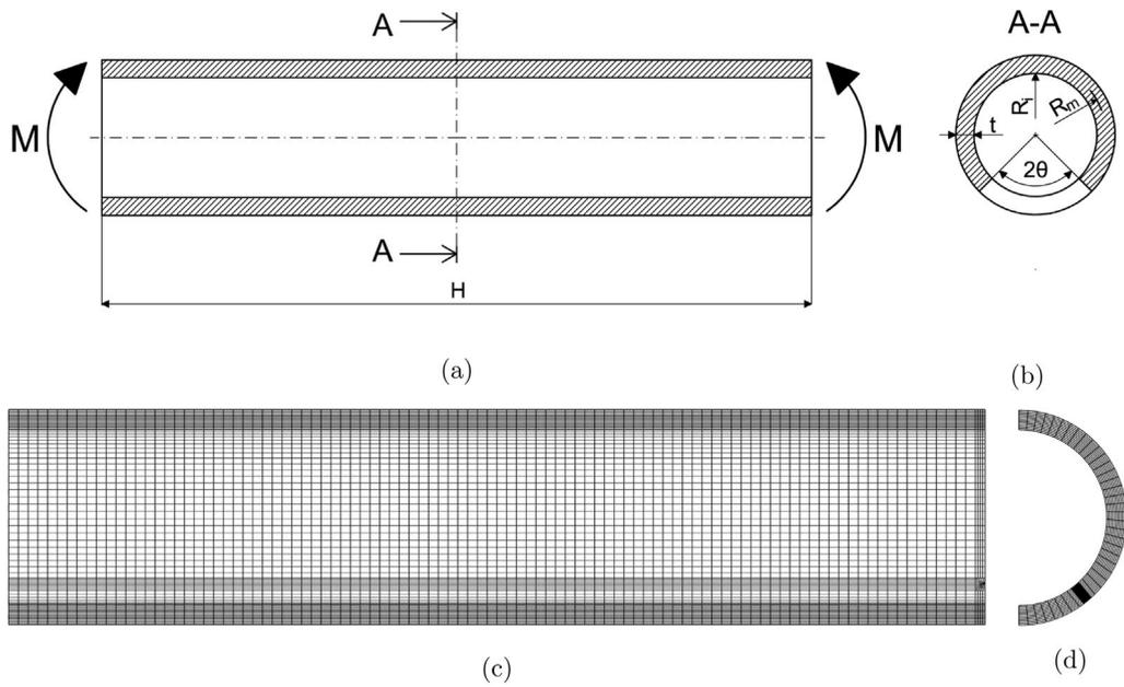
Fig. 3. Circumferentially through wall cracked (TWC) pipe with  $\alpha = 0.22$  (Table 6): (a) schematic view of pipe under pure bending moment, (b) pipe cross-section, (c) mesh view from inner surface, (d) mesh view from A-A direction.
