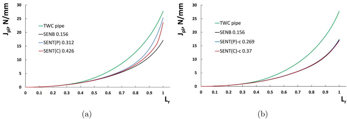
**Fig. 14.** TWC pipes and plane strain specimens using EPH material option: (a)  $J_{pl}$  values at limit load for plane strain specimens and TWC pipe, (b)  $J_{pl}$  values for TWC pipe, SENB and corrected SENT(P)-c, SENT(C)-c.
