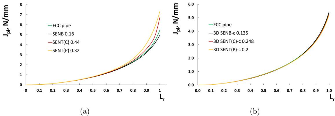
Fig. 17. FCC pipe and samples simulated using EPH material: (a) FCC pipe and plane strain samples, (b) FCC pipe and three-dimensional samples.
