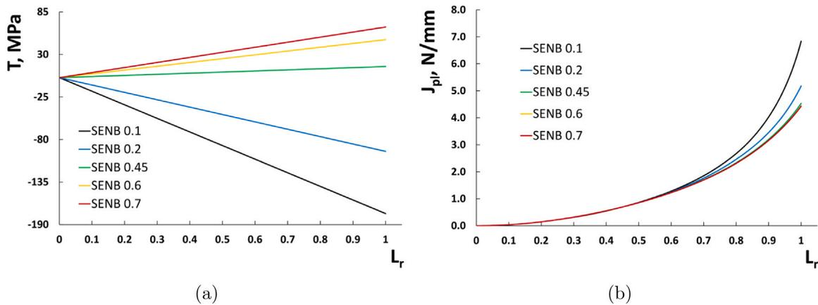
Fig. 8. The influence of  $T$ -stress on  $J_{pl}$  values in SENB specimens: (a) Different  $T$ -stress values for a fixed value of  $J_{el} = 3.6 \text{ N/mm}$  at  $L_r = 1.0$ ; (b)  $J_{pl}$  curves with EPH material for different constraint levels.
