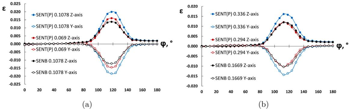
**Fig. 13.** Elastic-plastic strain distribution around the crack tip at the distance of 0.5 mm for SENB and SENT(P) samples: (a) SENB 0.1078, SENT(P) 0.1078 and SENT(P)-c 0.069, (b) SENB 0.1669, SENT(P) 0.336 and SENT(P)-c 0.294.
