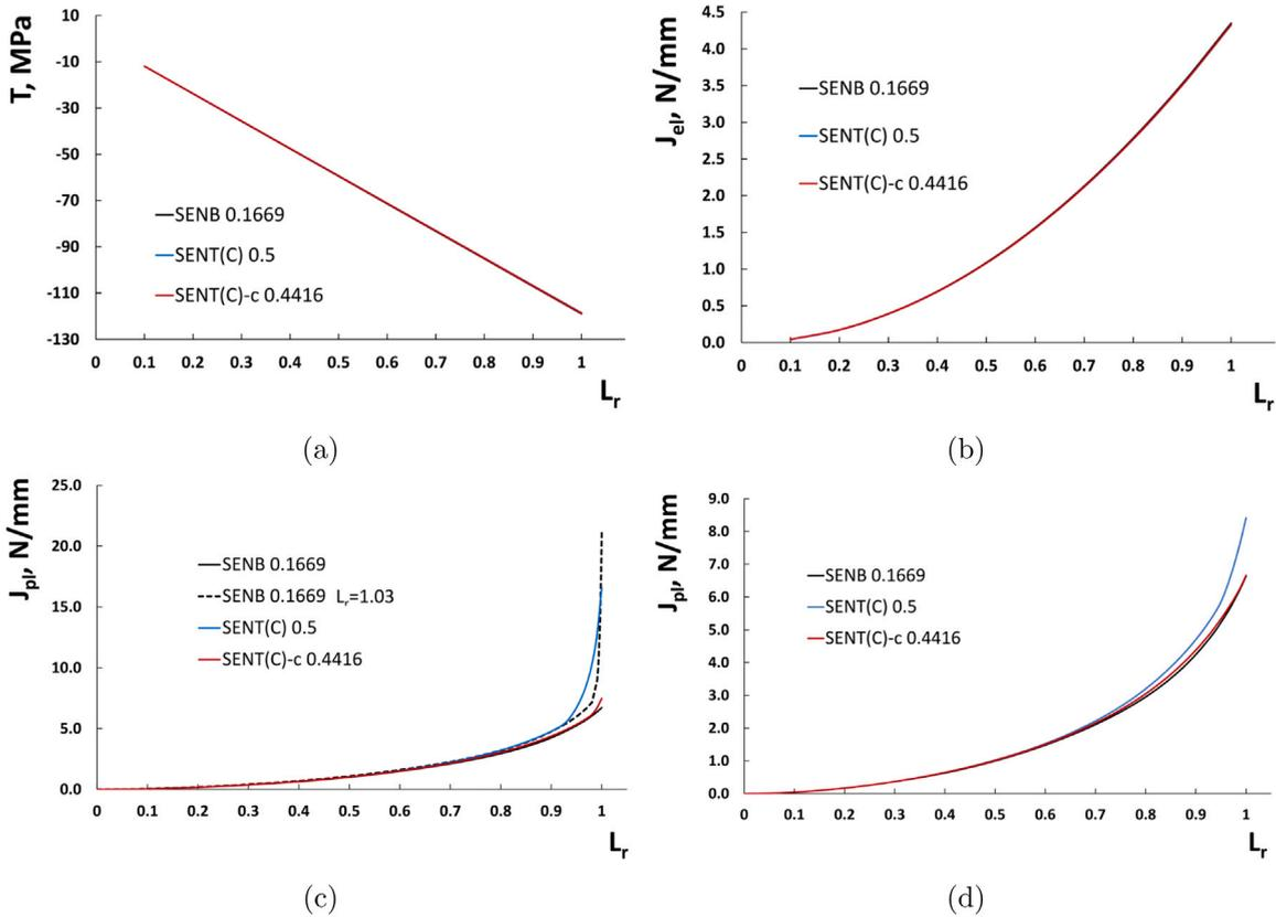
Fig. 10. SENB-SENT(C) deeper cracks. (a)  $T$ -stress values at limit load (b)  $J_{el}$  values at limit load (c)  $J_{pl}$  values at limit load using EPP material model (d)  $J_{pl}$  values at limit load using EPH material model.
