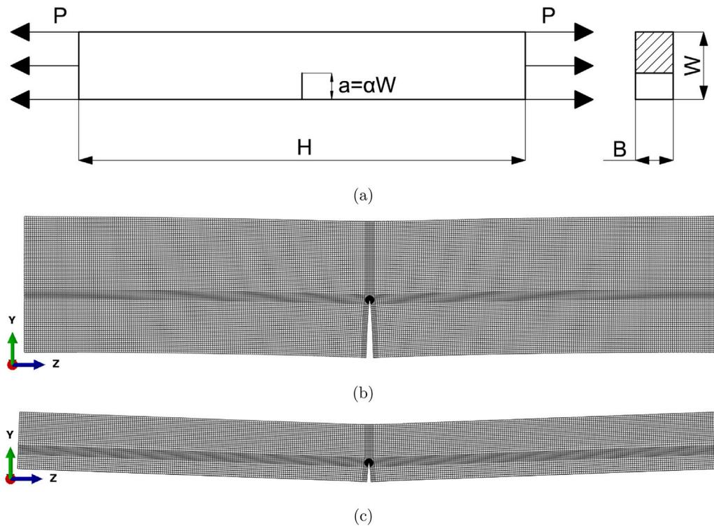
Fig. 2. Single edge notched tension specimen (SENT): (a) schematic drawing, (b) Finite element model of SEN(C) for  $\alpha = 0.426$  (see also Table 6), (c) Finite element model of SENT(P) for  $\alpha = 0.336$  (see also Table 5)
