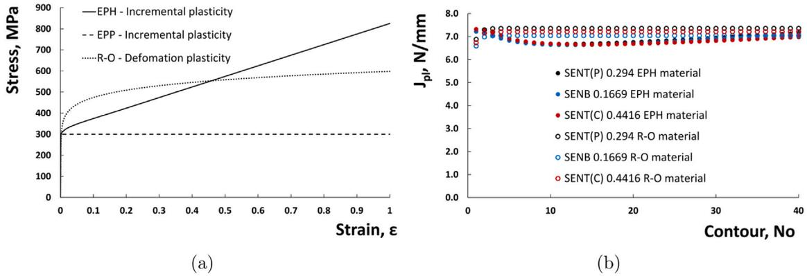
Fig. 6.  $J_{pl}$  values from incremental and deformation plasticity models: (a) stress–strain curves, (b)  $J_{pl}$  contour dependence curves of SENB and SENT specimens from Sections 6.3 and 6.4 at  $L_r = 1.0$  for R–O and EPH materials.
