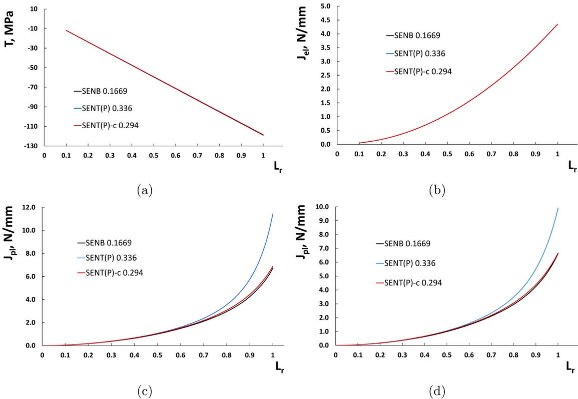
**Fig. 12.** SENB-SENT(P) deeper cracks. (a)  $T$ -stress values at limit load (b)  $J_{el}$  values at limit load (c)  $J_{pl}$  values at limit load using EPP material model (d)  $J_{pl}$  values at limit load using EPH material model.
