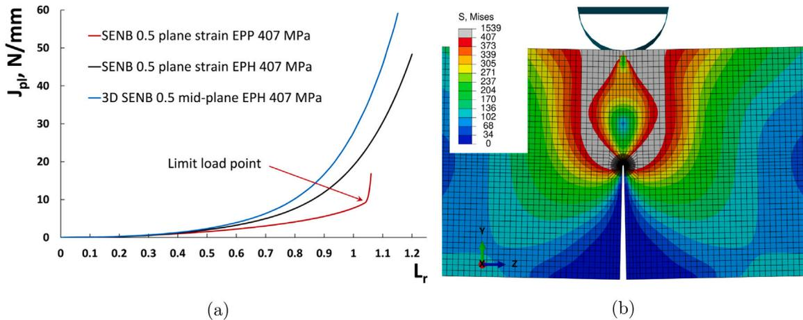
Fig. 15. Limit load analysis of SENB 0.5  $10 \times 10 \times 40$  mm specimen when  $\sigma_y = 407$  MPa: (a)  $J_{pl}$  curves under full plastic zone penetration into the ligament for an EPP and EPH materials with yield point offset, (b) full plastic zone (grey contour with values  $> 407$  MPa) penetration into the ligament.
