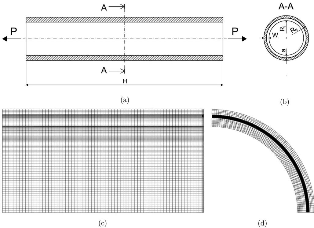
Fig. 4. Pipe with fully circumferential internal crack (FCC) with  $\alpha = 0.6$  (Table 8): (a) schematic view of pipe subjected to tension load, (b) pipe cross-section, (c) finite element model of 1/4 pipe segment, (d) cross-section mesh view.
