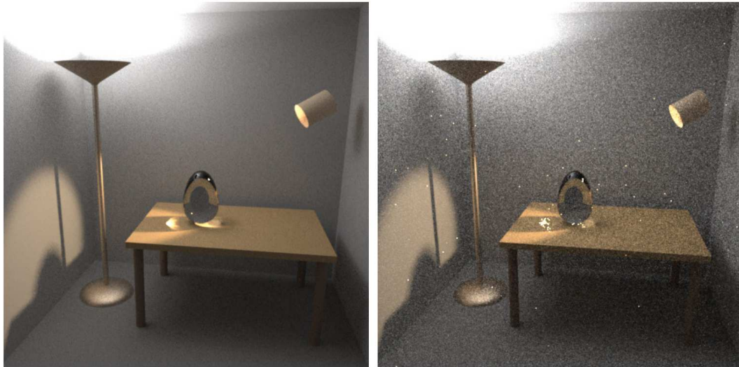
Figure 2.4: Bidirectional path tracing (left) vs. standard path tracing (right), equal-time comparison. BDPT clearly shows a better overall convergence of the image, with the issues in standard path tracing mainly caused by the specular object on the table. Caustics converge much quicker with BDPT, while a large amount of fireflies and noticeable noise are present when using standard path tracing in such a scenario. Images courtesy of (Veach and Guibas 1995b)
