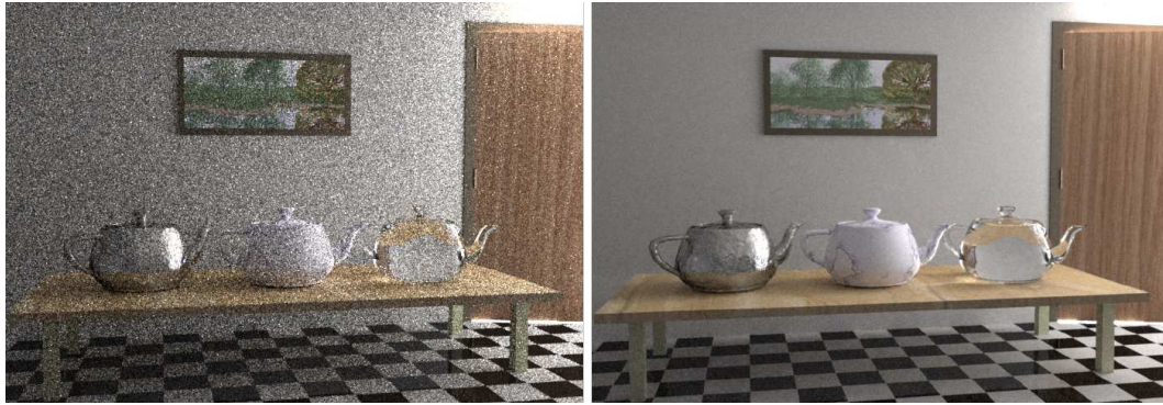
Figure 2.5: Bidirectional path tracing with 40 samples per pixel (SPP) (left) vs. Metropolis light transport with 250 mutations per pixel (right), equal-time comparison. The placement of the light source in this scene poses a challenge for path tracing, as light only comes through the slightly open door (according to the author, around 0.1% of the light from the adjacent room can enter through the door). The clear improvements in the MLT-based rendering mainly come from MLT’s ability to maintain path segments that connect the two rooms through the gap, while BDPT generates completely new subpaths with each iteration. Images courtesy of (Veach 1997)
