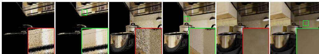
Figure 5.9: Interleaved comparison between filtering the first three accumulated bounces with traditional (red insets) and layered filtering (green insets). The image has been reconstructed with one sample per pixel after filling the cache with four samples per pixel just for the illustrated viewpoint. The utilization of local geometry information through layered G-buffers shows clear improvements in image quality. Filter weights for color and luminance differences have been adjusted in comparison to the weights chosen in the evaluation measurements.
