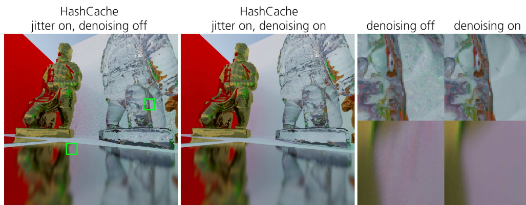
Figure 5.15: The effect of layered filtering for glossy and specular materials. The cache was filled irregularly over 128 frames at 1 spp for a random fly-through. (Left) Unfiltered image at 128 reconstruction samples per pixel. (Center) Layered filtering at 128 reconstruction samples per pixel. (Right) Magnified insets. It is clearly visible how the noisy illumination from the back wall is reflected in the glossy surface on the ground when layered filtering is deactivated. With layered filtering, the noise can be filtered in a separate layer and then be accounted for in the glossy reflection. For the refractive material on the right, a similar effect is visible: Refracted rays pick up the noisy cache values from the back wall when layered filtering is deactivated. With layered filtering turned on, this noise can be effectively filtered before it is propagated to preceding bounces. This allows for removing the noise locally without loss of details. An example for the individual layers being filtered is shown in Figure 5.9.
