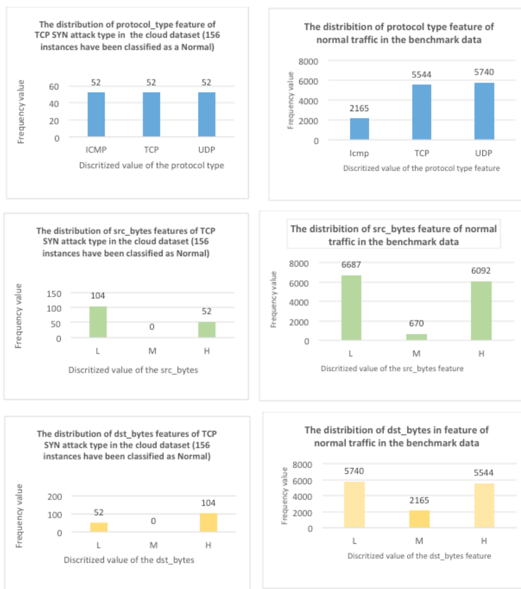
Figure 3.12 Distribution of TCP SYN attack instances that have been classified as normal instances in the benchmark data
