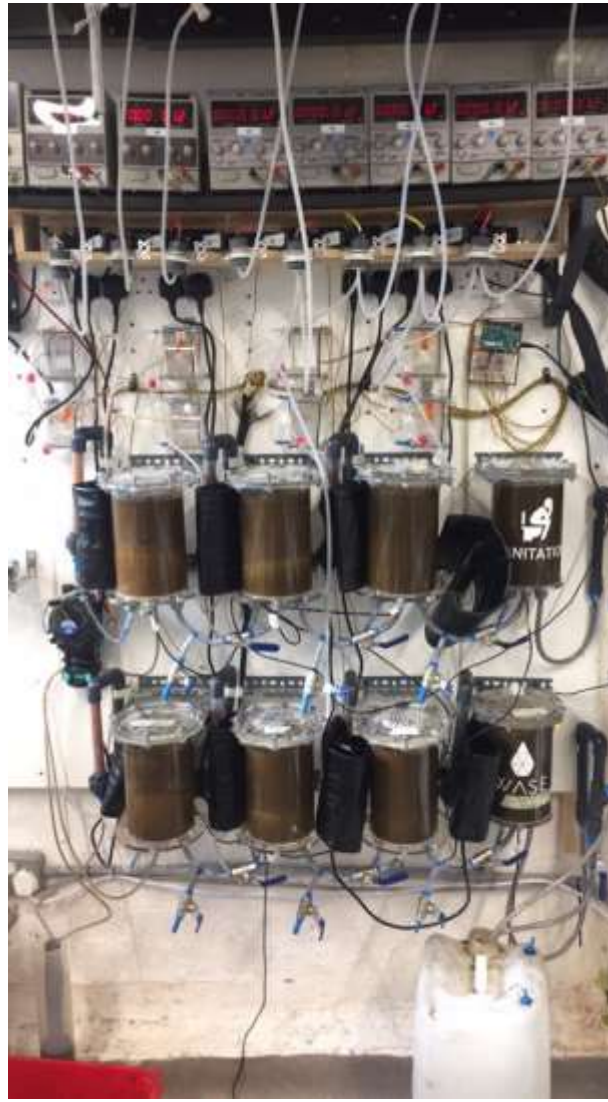
Figure 5-7: Brewery wastewater series (Duplicates) and batch EMR and AD analysis – Heating jackets removed
