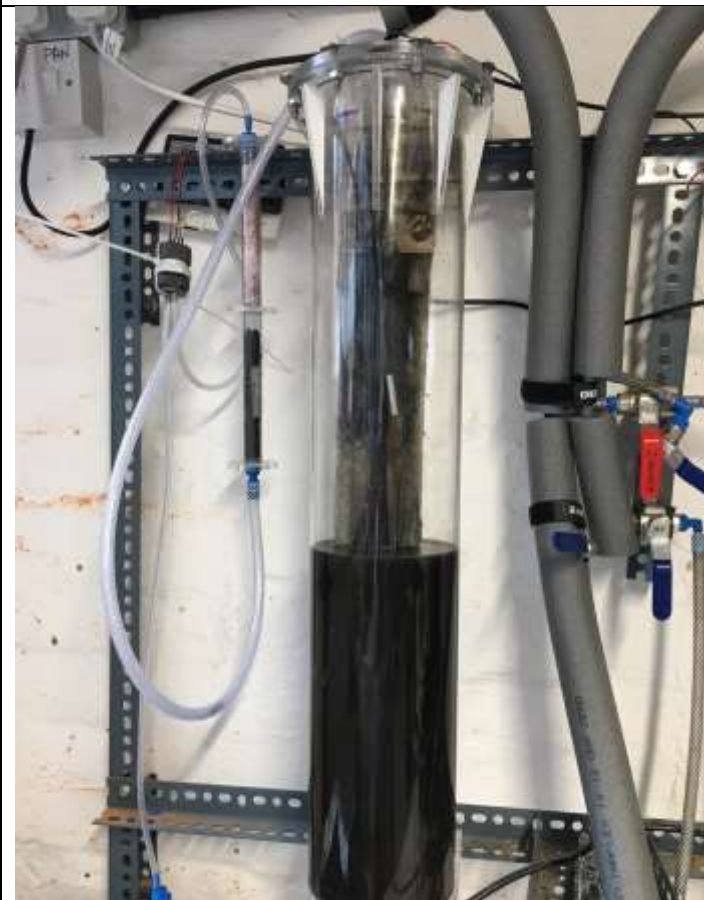
Figure 13-26: 7L AD and EMR test system
