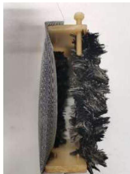
Figure 5-3: Carbon Brush Anode & Stainless Steel Pocket & GAC Cathode - Side View
