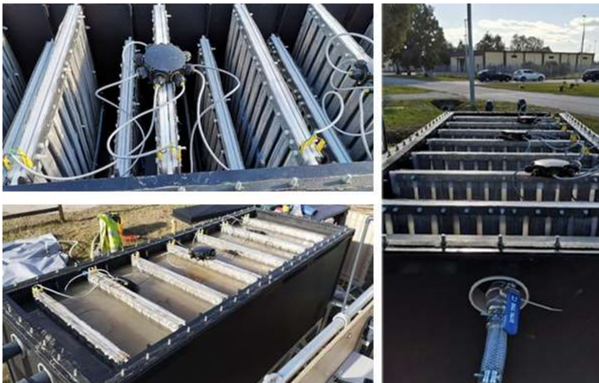
Figure 9-10: EMR Pilot Electrode Placement Images
