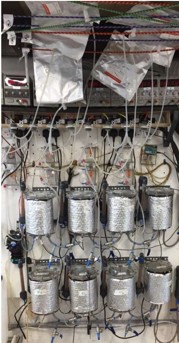
Figure 5-6: Brewery wastewater series (Duplicates) and batch EMR and AD analysis – Experimental setup
