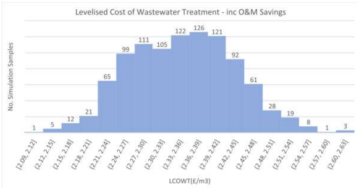
Figure 10-14: Levelised Cost of Wastewater Treatment with O&M minus biogas value
