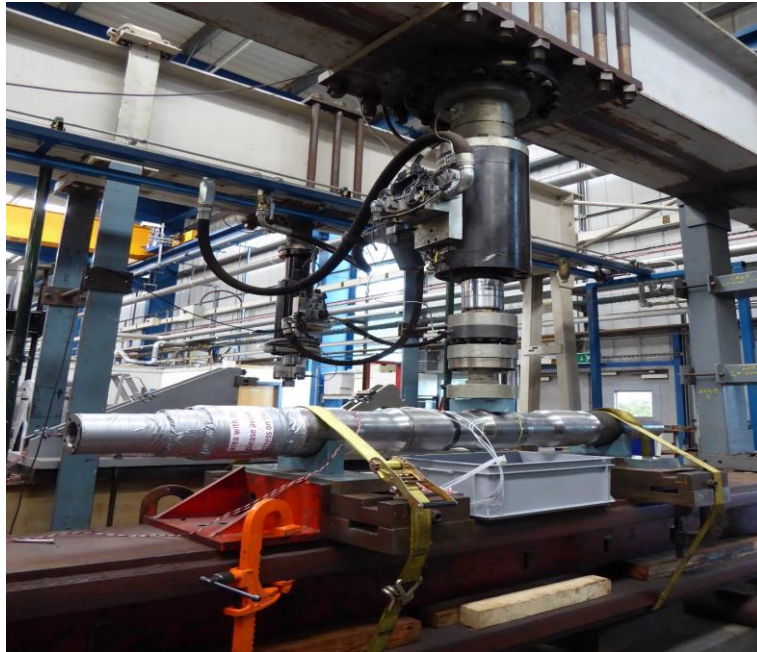
Figure 3-45 Pit formation Method 4 set up
