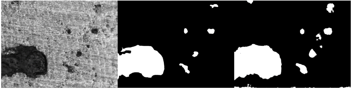
Figure 7-30 Deep Learning pixel-wise UNet-Vgg16 performance on Image A925-17
