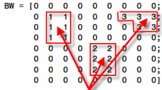
Figure 5-27 Showing Labelled connected component in an image [138]
