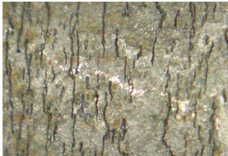
Figure 2-5 Typical example of micro-cracks in an image taken from an axle
