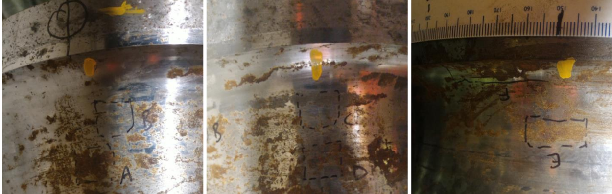
Figure 1-2 Example of manual visual assessment and pit counting
