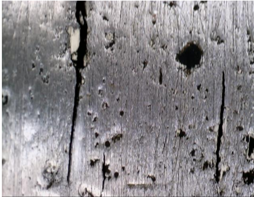
Figure 2-9 Magnetic particle inspection (MPI) example
