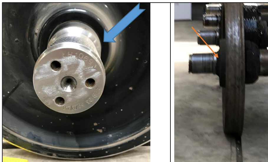
Figure 4-26 Site image showing location of suspected corrosion on axle
