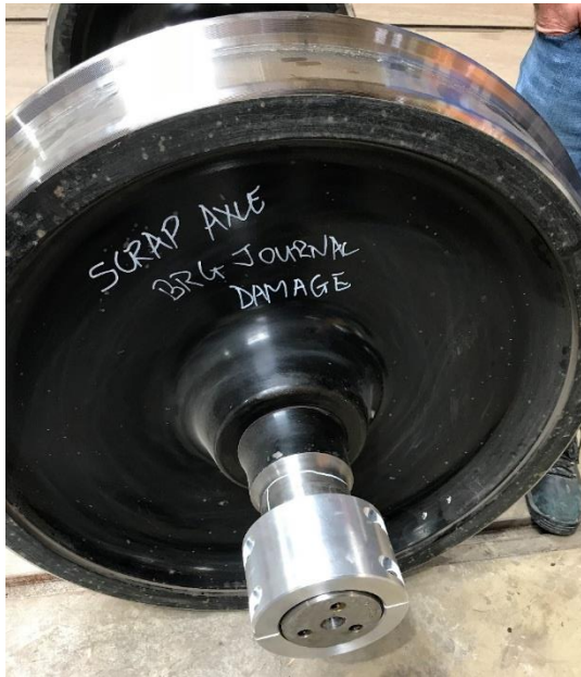
Figure 4-27 Site image of Sleeve to adapt to journal diameter
