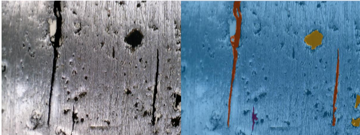
Figure 4-40 Image labeller showing ground truth marked with separate classes
