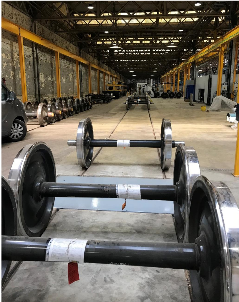
Figure 4-25 Site images of Freight (ballast train) axles in depot for inspection
