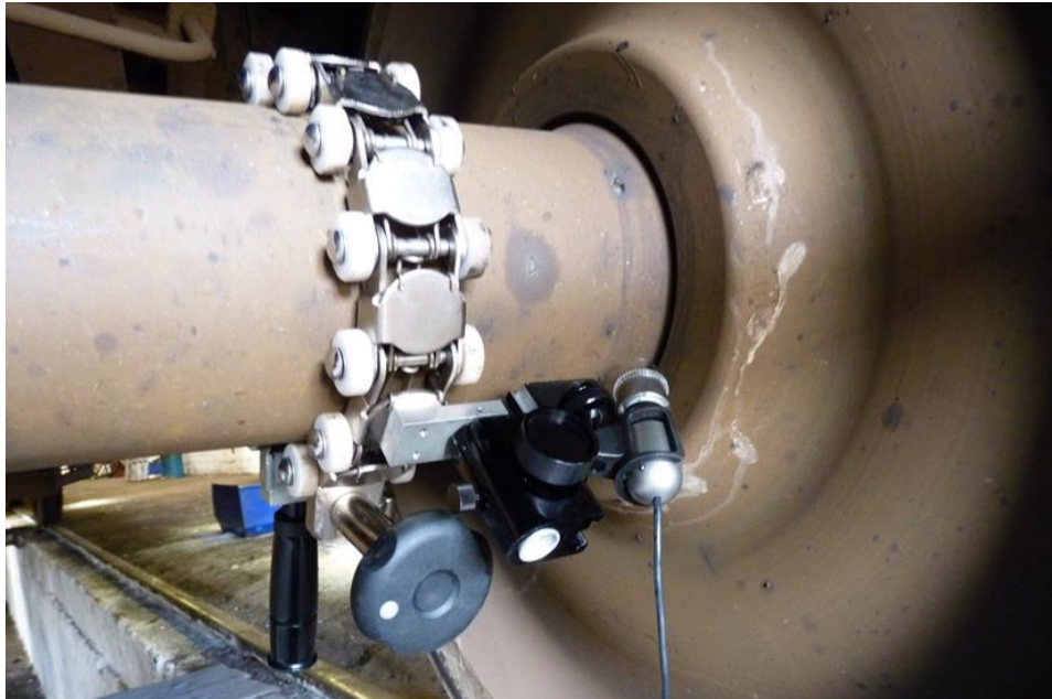
Figure 3-27 Manual chain scanner along with the microscope and its holder
