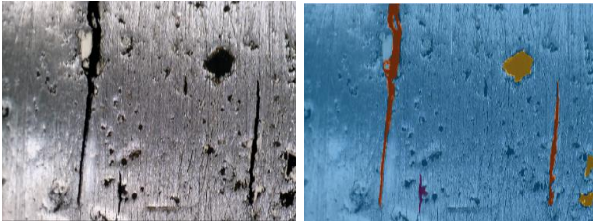
Figure 4-37 Image showing pits, cracks and pit-to-cracks marked by Image Labeller
