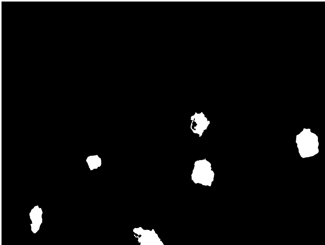
Figure 5-70 Flaw measurement detected by Watershed algorithm on same image
