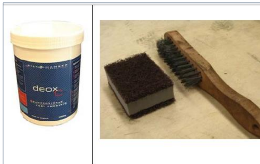
Figure 3-33 Chemical rust remover and abrasives used
