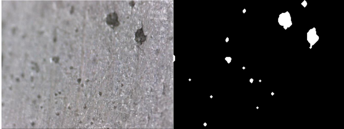
Figure 5-65 FCM Gaussian outcome on B514-16 showing resultant binary image
