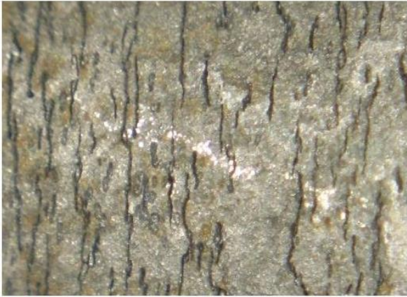
Figure 3-34 Sample of micro-cracks on an axle
