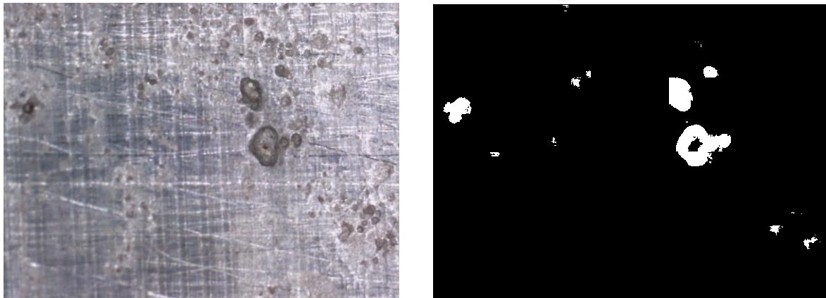
Figure 7-21 Deep Learning UNet model showing results for less pitted sample image
