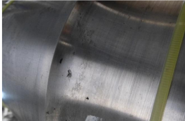
Figure 4-7 Sample axle that needs to have track markings to monitor flaw positions
