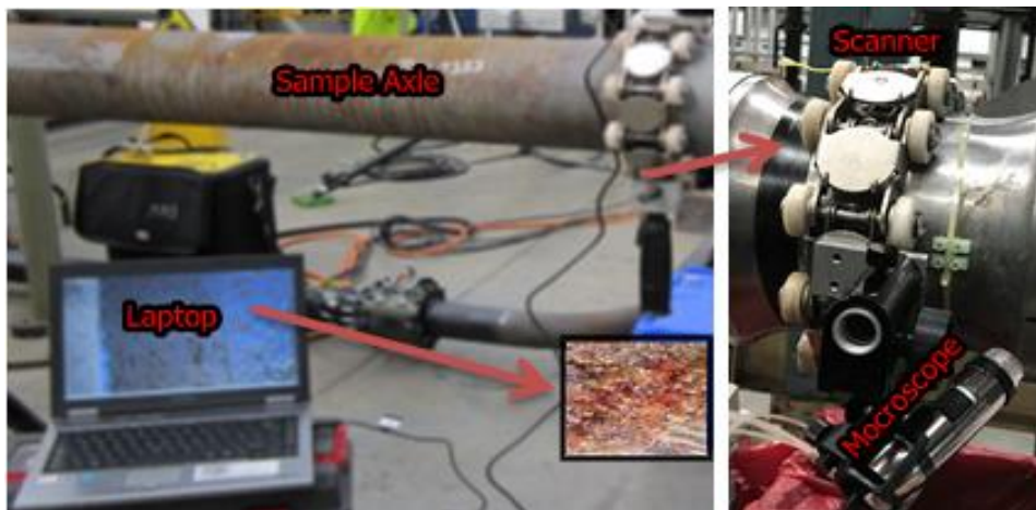
Figure 3-49 Setup of the data collection system with manual scanner
