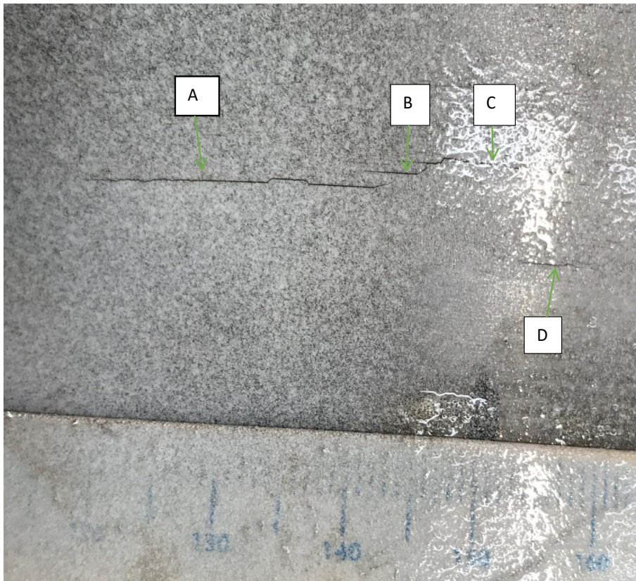
Figure 3-8 Nomenclature for cracks at 12 o'clock
