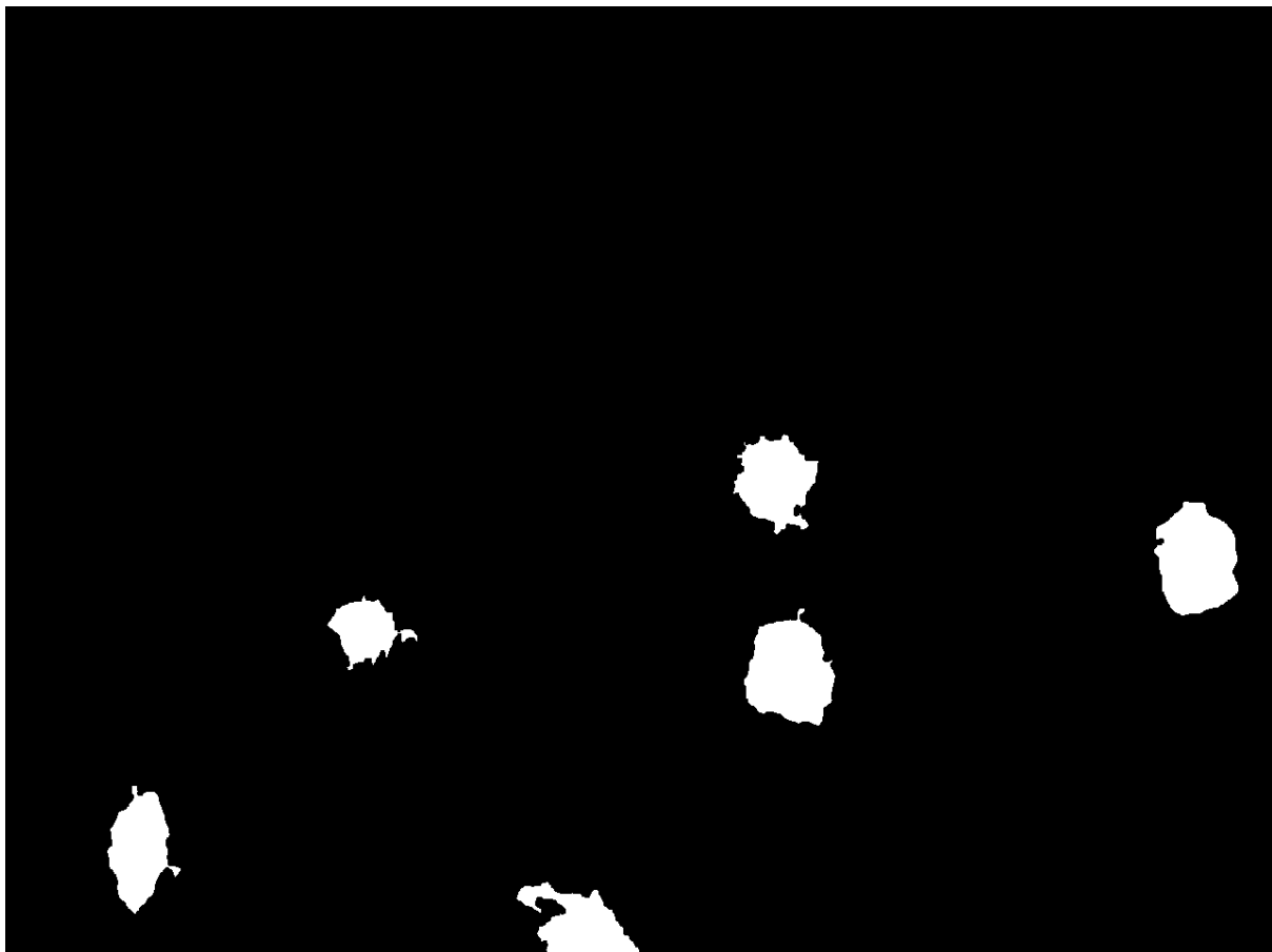
Figure 5-71 Flaw measurement detected by Morphological Method on same image
