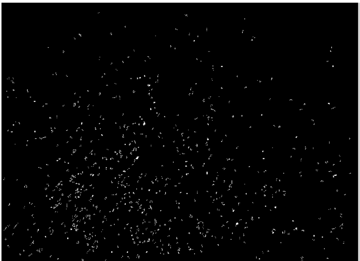
Figure 5-15 Result of real original axle image after applying 'Sobel' edge detector
