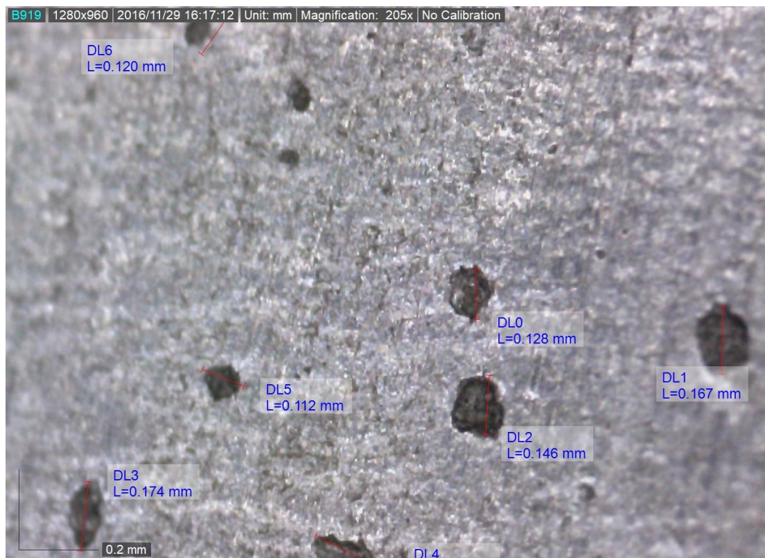
Figure 5-68 Manual measurements made for labelling the test image
