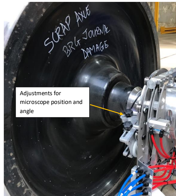
Figure 4-28 Site image of Sleeve to adapt to journal diameter with the scanner mounted
