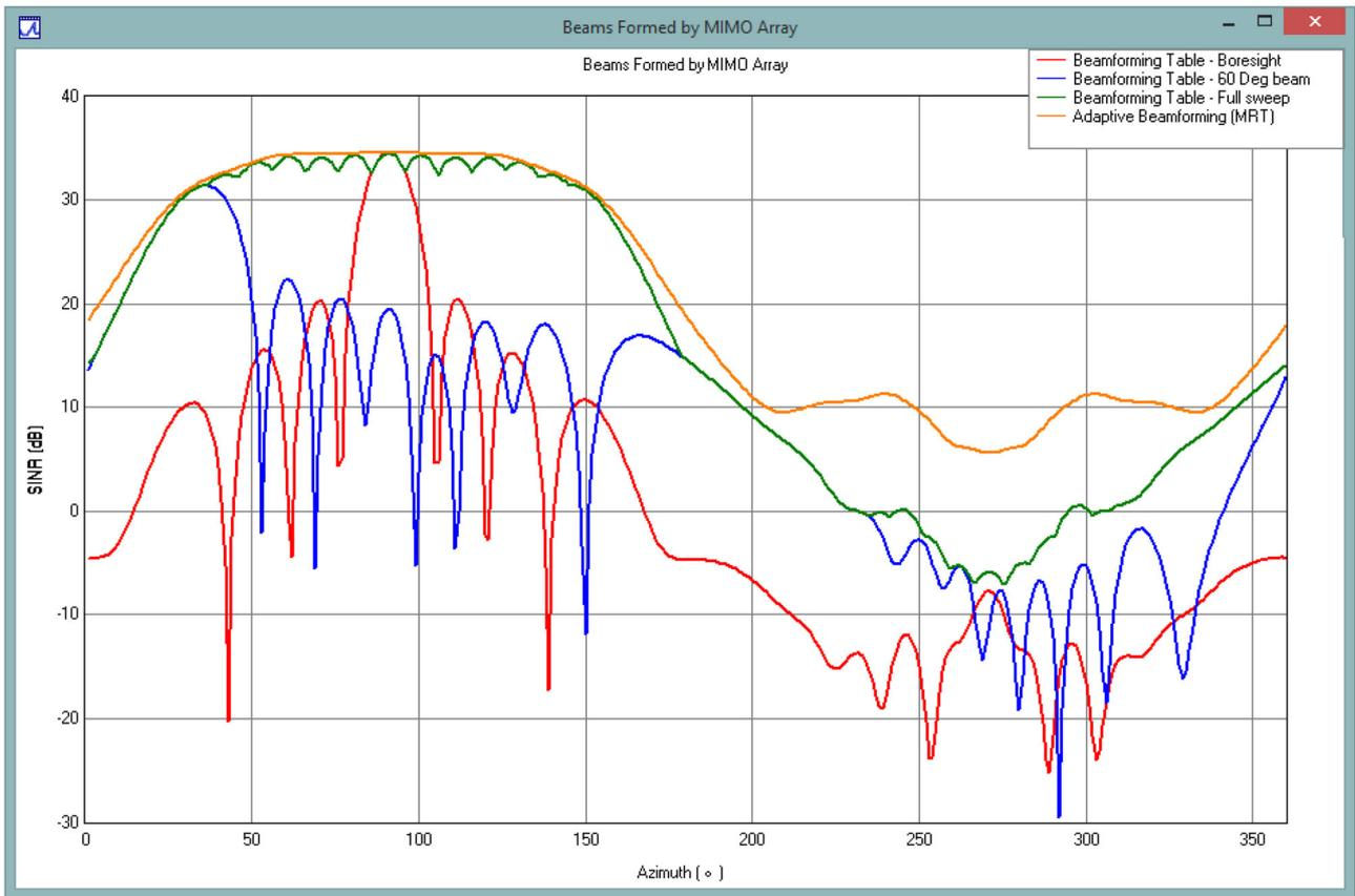
Fig. 11 SINR against Azimuth at various radiation patterns
