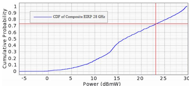
Fig. 8 5G MIMO antenna CDF of EIRP
