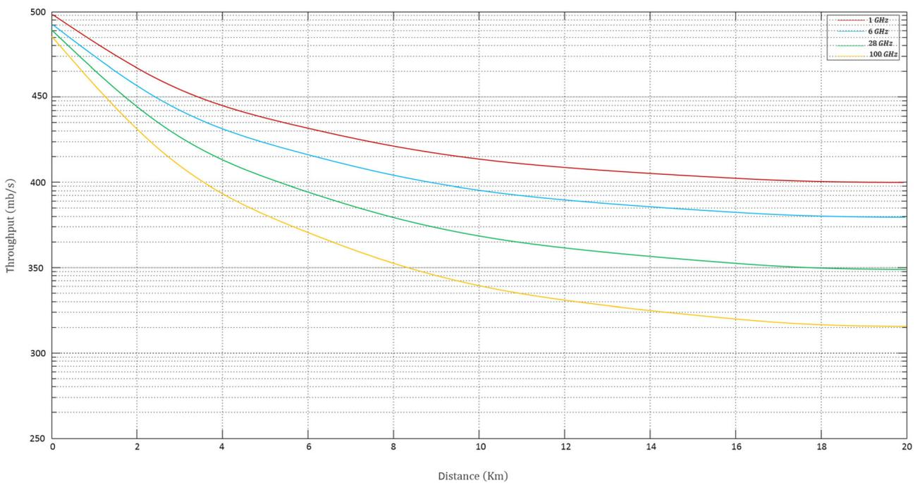
Fig. 10 Throughput against distance at various frequencies
