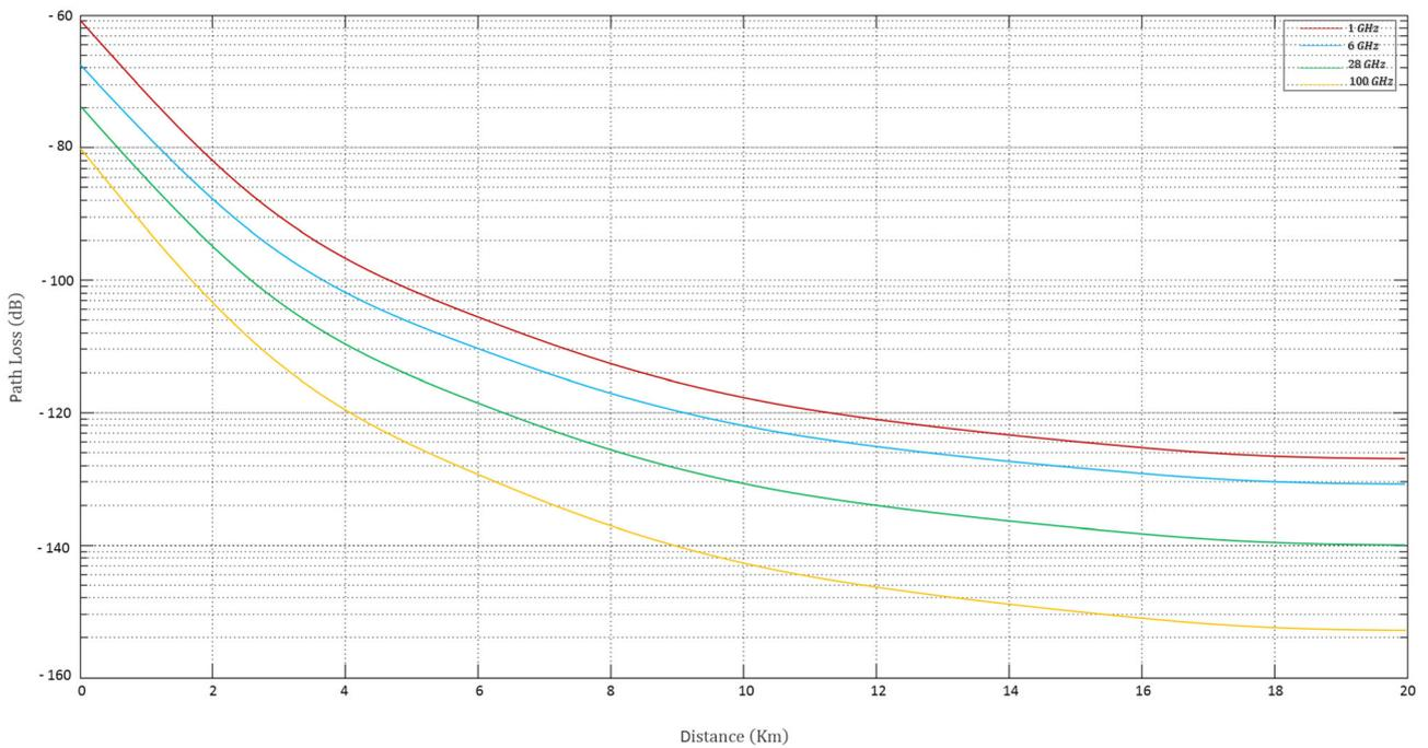
Fig. 9 Path loss against distance at various frequencies
