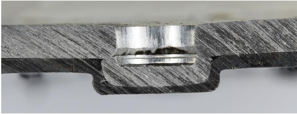
Figure 47 – Cross section of a clinch joint. Failure of neck can be seen.
