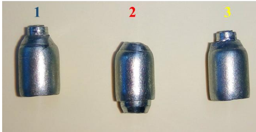
Figure 35 – Rivets from TSS with different shearing behaviour. In Samples 1 and 3, the mandrel did not retract while in Sample 2 it is retracted displaying a different loading behaviour in TSS curves.
