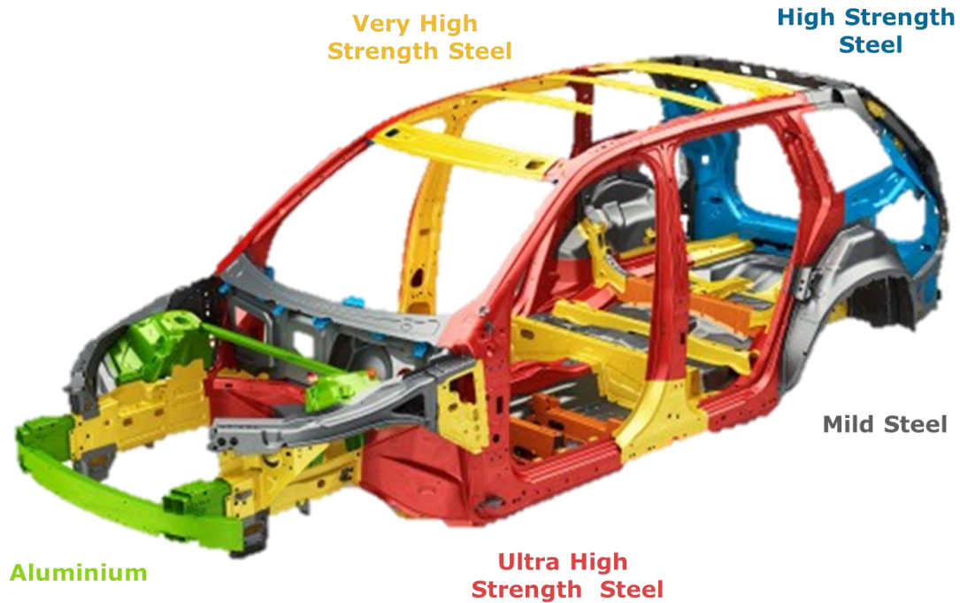
Figure 2 – Dissimilar material BIW of a prototype from Volvo XC90
