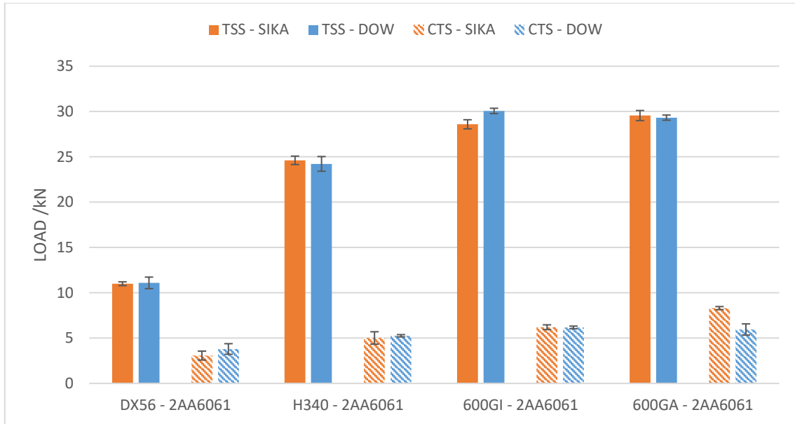
Figure 29 – TSS and CTS results for the adhesive bonded samples with Sika (orange) and Dow (blue) of joints made with 2AA6061 and different steels.
