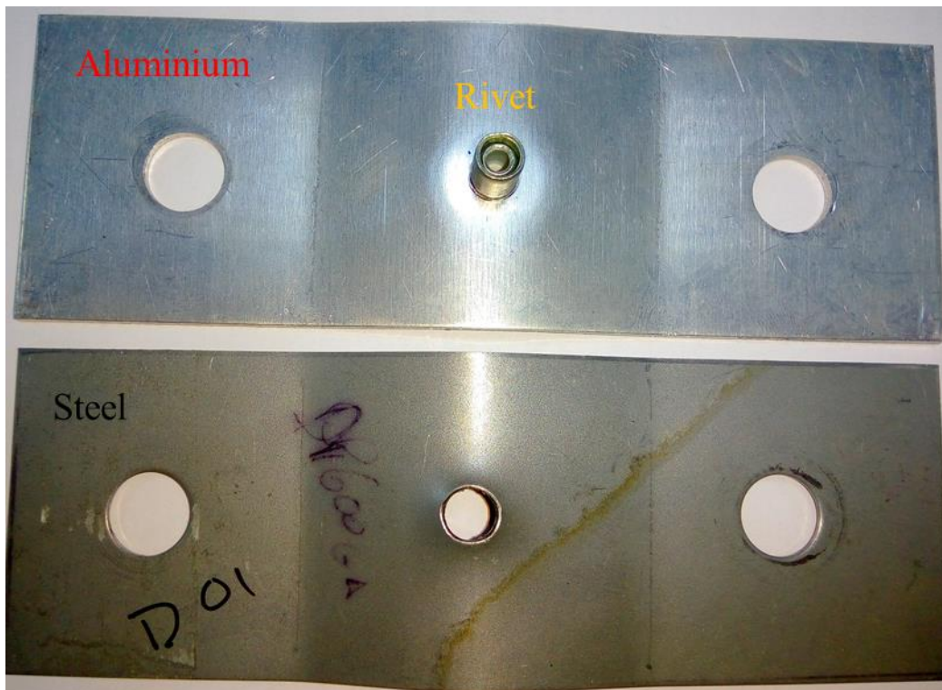
Figure 36 – Tested cross tension specimen. Failure associated with material deformation around the centre hole in the steel
