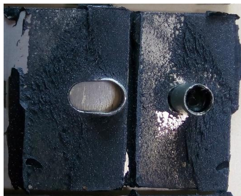
Figure 40 – Adhesive cohesion and adhesion failures followed by interlock failure
