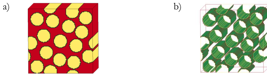
Figure 4.1.5 Mesoscale model with fibre-matrix debonding damage mechanism a) the whole model, b) elements with changed properties – debond layer
