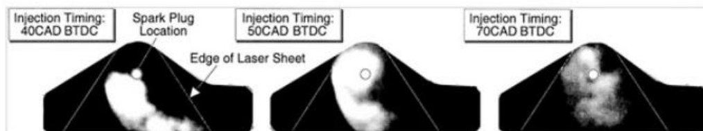
(b) Comparison of Gasoline LIF Distributions in the Cases of Different Injection Start Timings (With Reverse Tumble, Imaging Timing: 15CAD BTDC).
