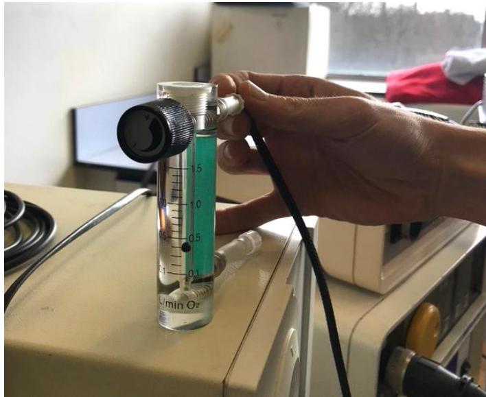
Figure 3.8.1 Manual dry-gas flow-meter. The black float indicated the rate at which air was extracted via the black sample tube. Note that the angle from which the picture was taken does not accurately show the flow rate.
