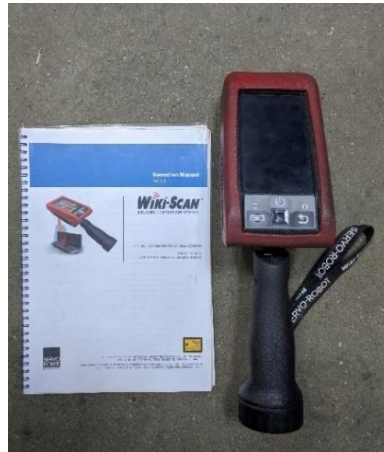
Figure A.1 Wiki-scan welding inspection system
