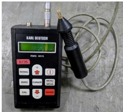
Figure 3.10 The alternating current potential drop (ACPD) device used for crack depth monitoring.
