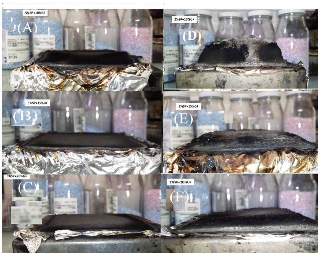
Figure 6-9 : Photograph of char residue after CCT for low loading sepiolite 2%SP (left) and higher sepiolite 5%SP(right) with GF 10%,15%,20%
