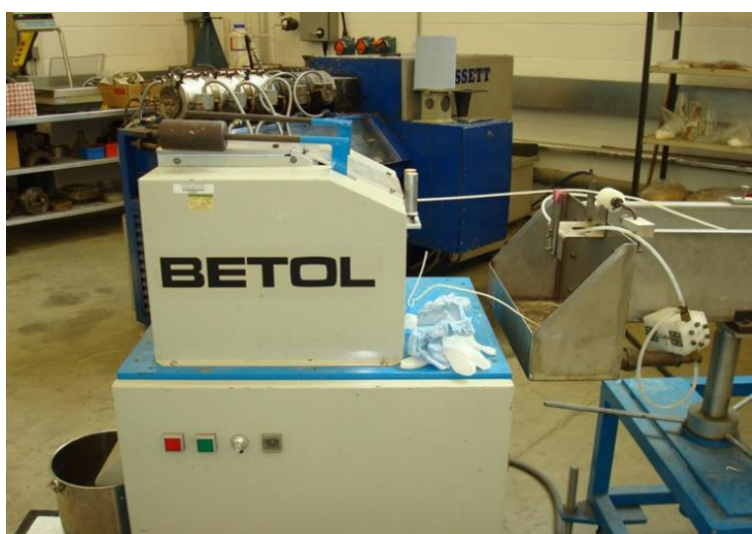
Figure 3-7: Twin screw extruder co-rotating intermeshing
