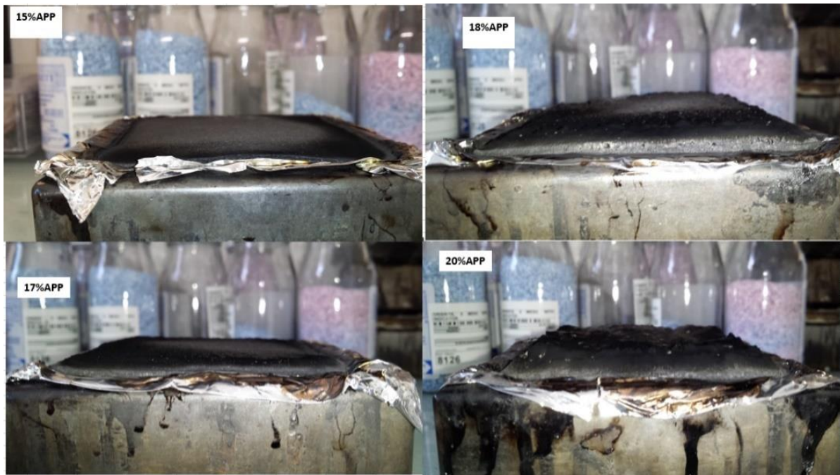
Figure 5-9: Top view photographs of char residue after CCT with different IFR contents: (a) 15% IFR, (b)17% IFR, (c) 18% IFR and (d) 20% IFR
