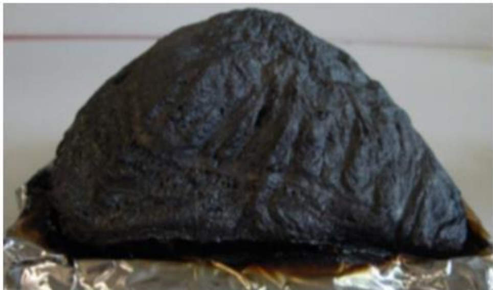
Figure 2-17: Intumescent char protection layer formation
