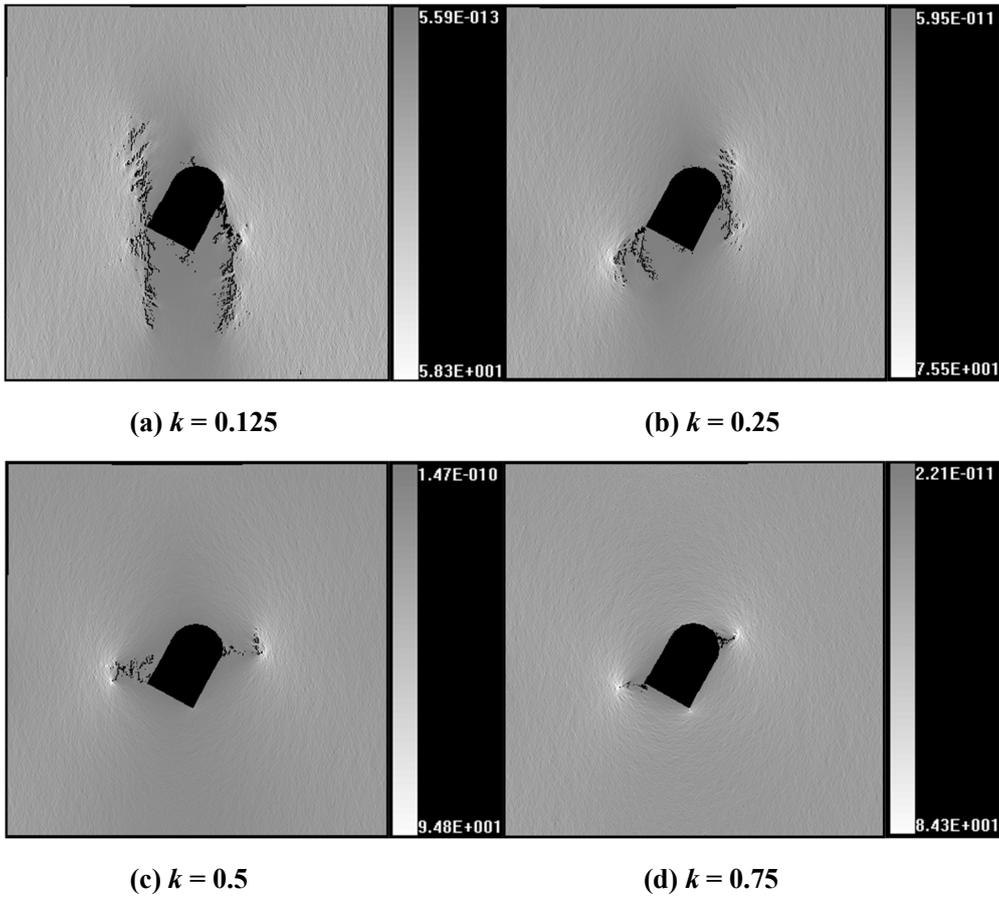
**Fig. 10** Shear stress contour with the lateral pressure coefficient  $k$  changing by simulation (Unit: Pa)
