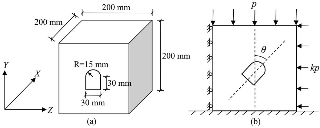
**Fig. 2 The physical model (a) model size and (b) loading conditions**
