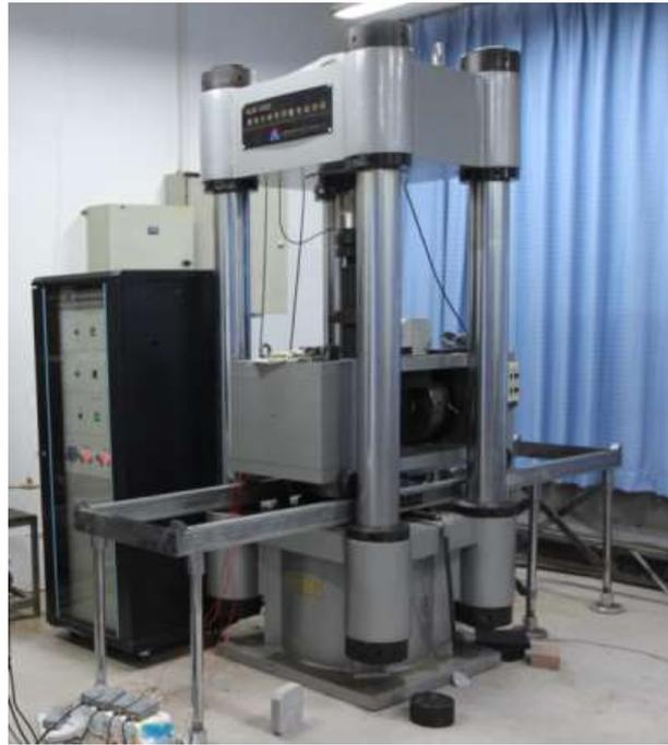
**Fig. 1 RWL-3000 servo-controlled testing machine**
