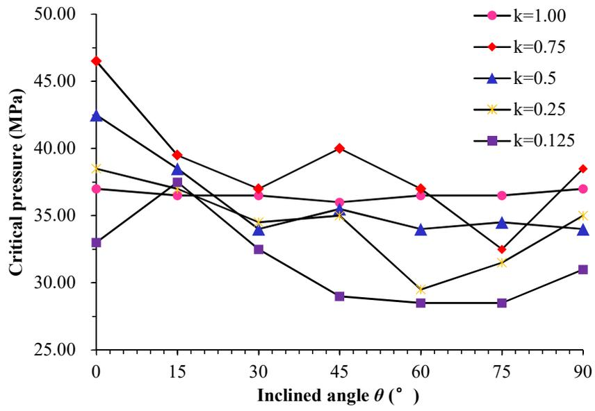
**Fig. 11 Critical pressure curves of horseshoe-shaped tunnel model**
