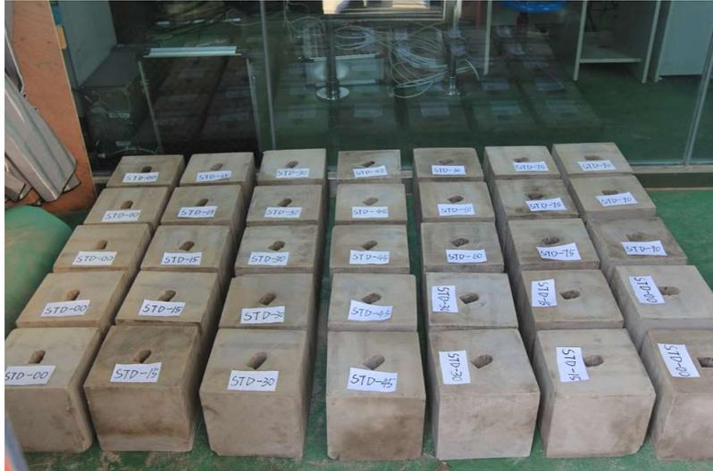
**(a) Physical models made of cement mortar**
